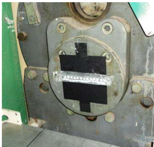
Figure 2. TLD dosimeters placed at the exit of the HK1 collimator for irradiation.
