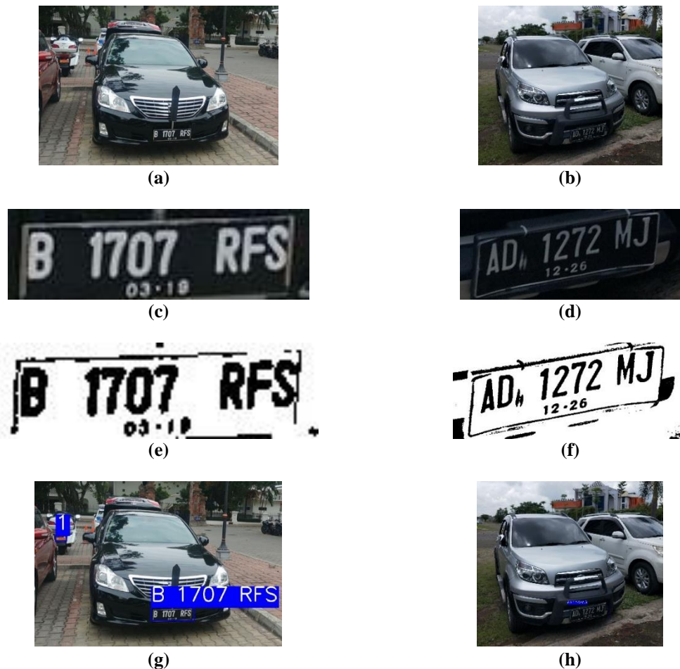
Figure 5. (a)-(b). images original; (c)-(d). bounding box detection; (e)-(f). digital images processing; (g)-(h). integration algorithm results
