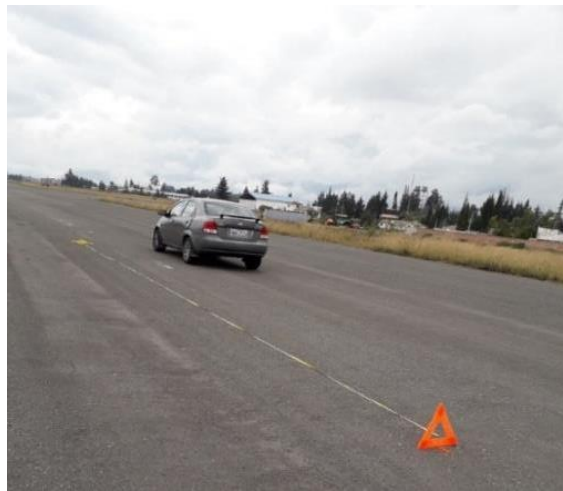
Figure 14 Braking distance at 50 km/h
