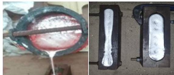
Figure 3: Pouring molten metal.
