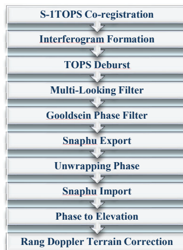
Figure 3. The standard Interferometry Processing workflow within SNAP software
