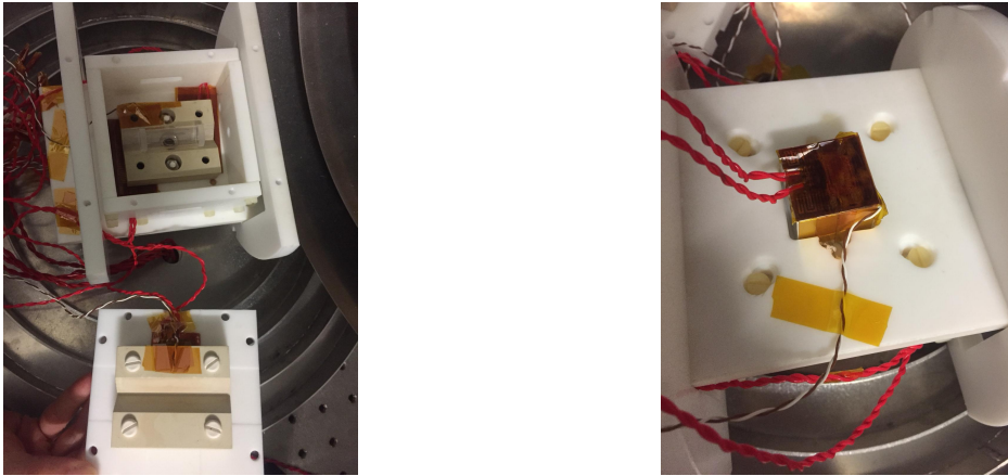
Figure 6.1.: Heater structure (a) ceramic structure of the main part (b) stem oven
