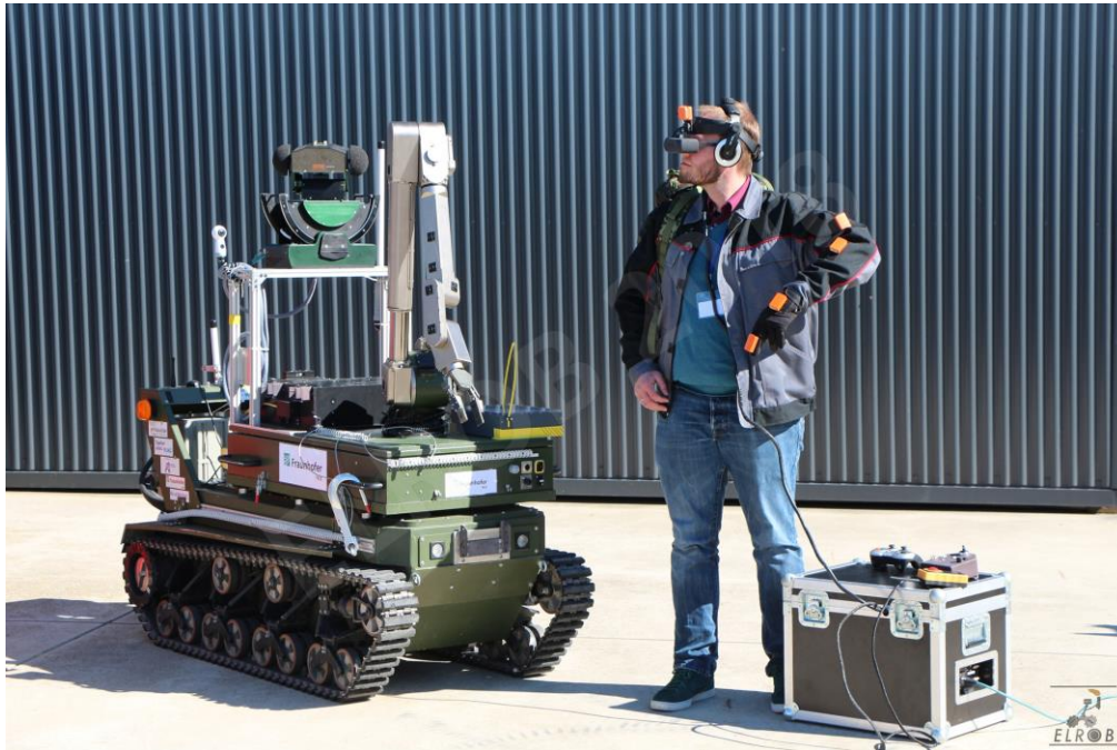
Figure 10. Mapping of human arm movement to a movement of the manipulator; stereoscopic vision and tracking of head movement
