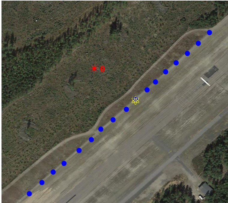
Figure 15. UGS passing a source and marking the nearest point to source on the road. The coordinates (Long, Lat) at the measurement point of the maximum doserate should be reported immediately after passing the source (< 10 s)
