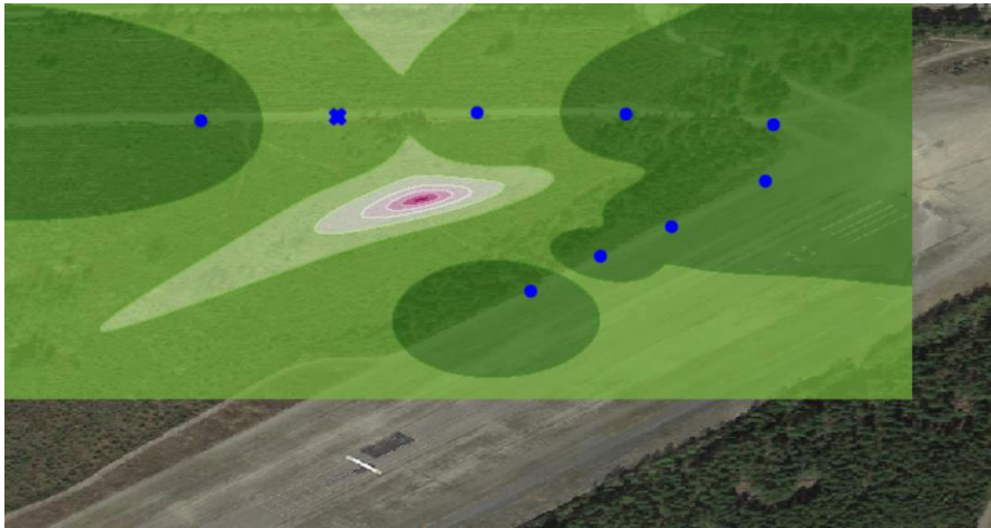
Figure 22. Source localization by one UGS using spectrometric data. The area of interest is correctly localized and the nuclide identified as Se-75 with estimated activity 9.1 \times 10^{10} \text{ Bq} \pm 28\%
