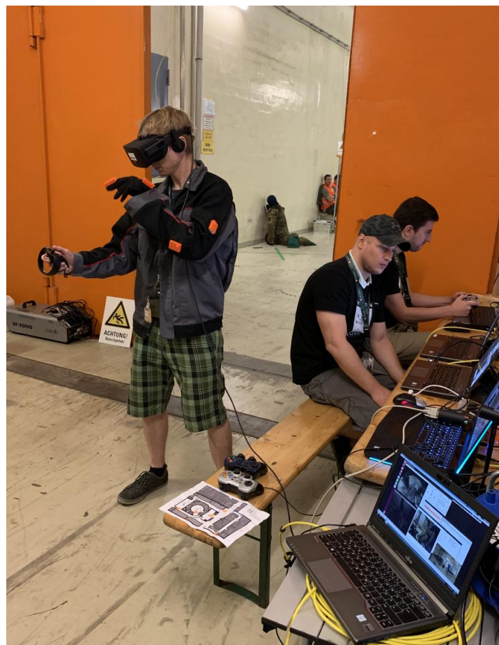
Figure 11. Human-arm to robot-arm mapping but with VR/AR assistance using 3D model of the facility generated by laser scanner and video camera (in Zwentendorf NPP)
