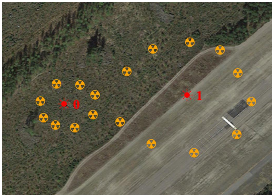
Figure 19. Isocurve in an unknown radiation field; the markers dropped by a robot refer to a doserate of about 10 \mu\text{Sv/h} (isocurve criterion). The markers form an asymmetrical pattern. Conclusion: the area of interest seems to contain two sources. In fact, this scenario contained a Cs-137 source with activity of 5 \times 10^{10} \text{ Bq} and a Co-60 source with activity of 1 \times 10^{11} \text{ Bq}
