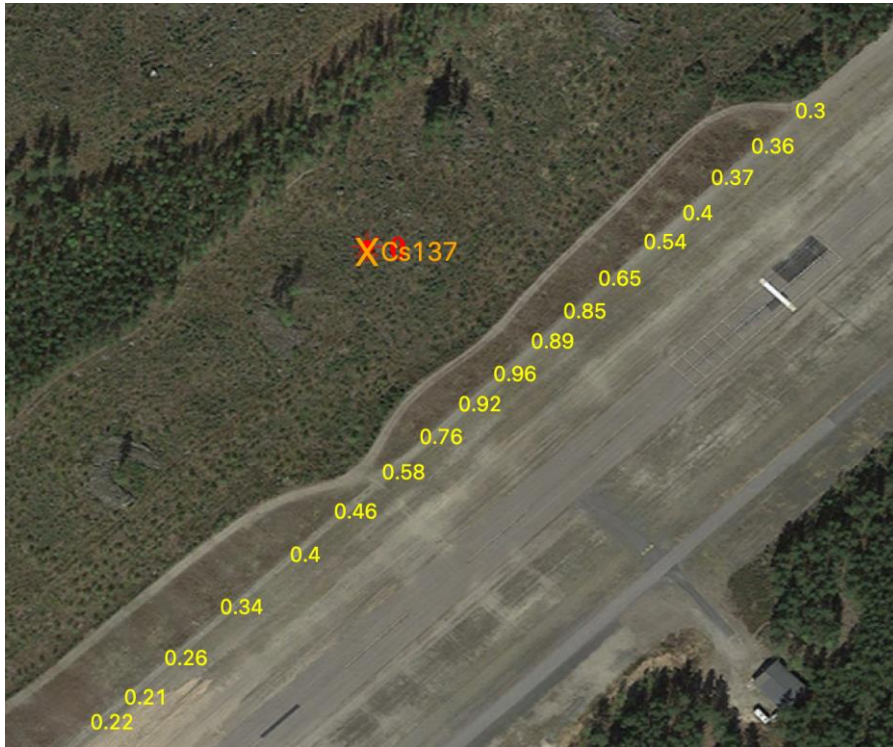
Figure 17. Most likely source location X and related activity calculation (symmetry issues omitted, see Figure 16). Activity estimation using spectrometric data was performed simultaneously with the source localization analysis giving 5 \times 10^{10} \text{ Bq} \pm 23\% for Cs-137. The measured dose rate is marked on the road ( \mu\text{Sv/h} ) passed by the UGS
