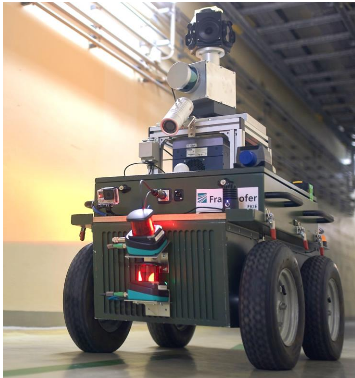
Figure 7. FKIE robot used for Zwentendorf NPP exploration
