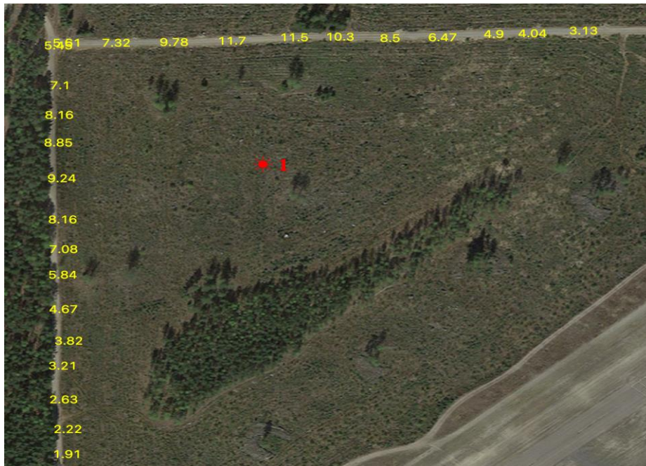
Figure 20. Doserate measured by two robots moving perpendicular to each other. The location of the source can be estimated from the maxim reading on both axes (see Figure 21)
