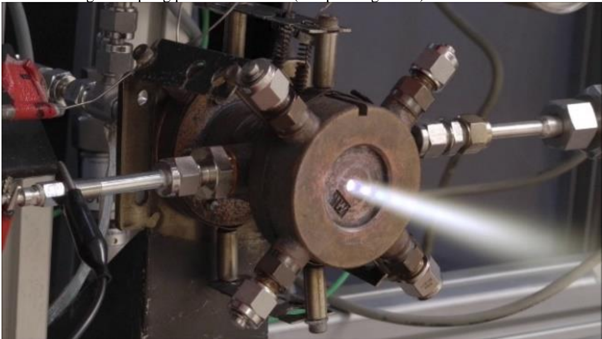
Figure 38: Experimental thruster during hot firing (liquid propellant ROF=6.8)
