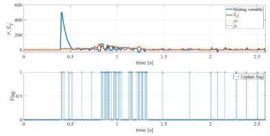
Fig. 11 Sliding variable and controller update flag of the ET- NCS
