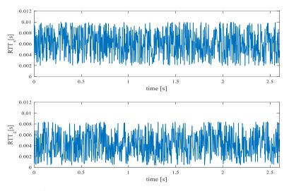
Fig. 7 Measured RTT<sub>s</sub> and RTT<sub>c</sub> values of the NCS network
