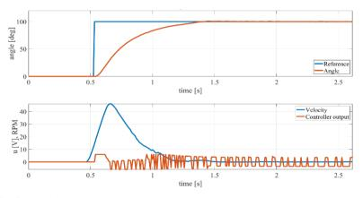
Fig. 8 Tracking capability, RPM value, and  $v_{\tau\tau}$  controller output of the TT- NCS
