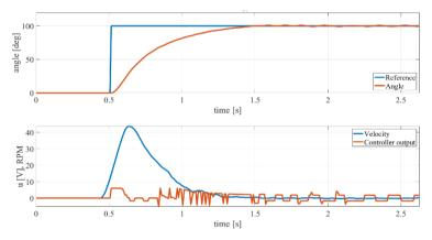
Fig. 10 Tracking capability, RPM value, and  $v_{ET}$  controller output of the ET- NCS
