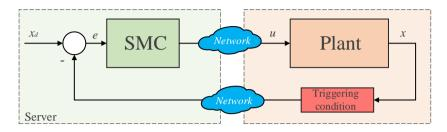
Fig. 2 ET-SMC feedback configuration
