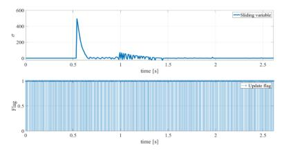
Fig. 9 Sliding variable and controller update flag of the TT- NCS
