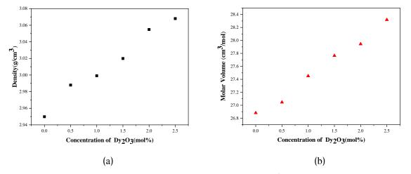
Figure 2 (a) Variation of density ( $\rho$ ) and (b) molar volume ( $V_M$ ) for the Dy<sup>3+</sup> doped ZnO-SrO-B<sub>2</sub>O<sub>3</sub> glass.
