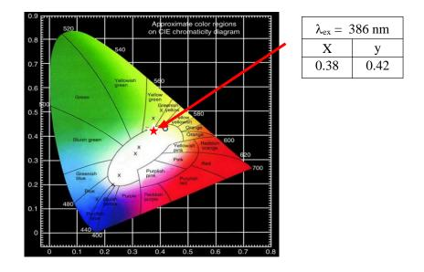
Figure 8 CIE chromaticity coordinates of ZnO-SrO-B<sub>2</sub>O<sub>3</sub> glass at different Dy<sub>2</sub>O<sub>3</sub> contents.
