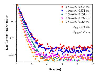
Figure 7 Luminescence decay profiles of the  ${}^{4}F_{9/2}$  level of  $Dy^{3+}$  in ZnO-SrO-B<sub>2</sub>O<sub>3</sub> glass at different  $Dy_{2}O_{3}$  contents.
