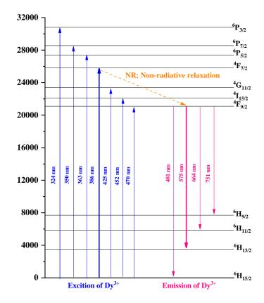
Figure 6 The Partial energy levels diagram of the  $Dy^{3+}$  ions in the ZnO-SrO-B<sub>2</sub>O<sub>3</sub> glass.
