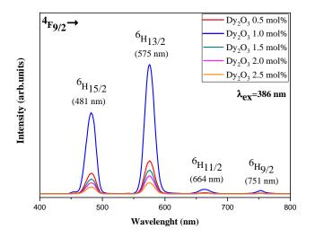
Figure 5 The emission spectra of the ZnO-SrO-B<sub>2</sub>O<sub>3</sub> glass at different Dy<sub>2</sub>O<sub>3</sub> contents.
