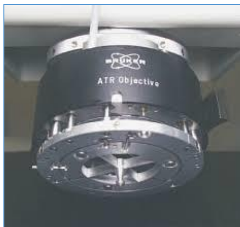
Figure 4.4 ATR objective with germanium crystal.
