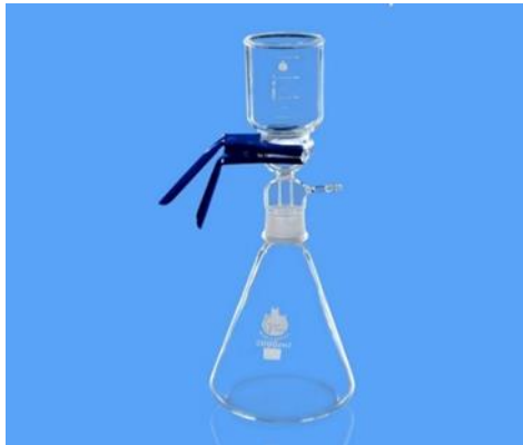
Figure 3.10 Glass filtration assembly.
