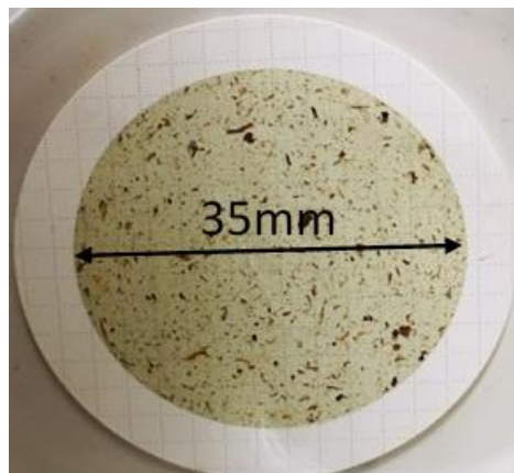
Figure 3.11 Filter paper with particles.
