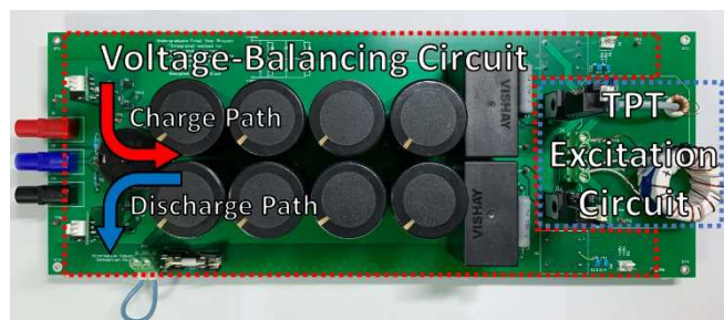
Fig. 5. TPT integrated testbed with new voltage-offsetting circuit included
