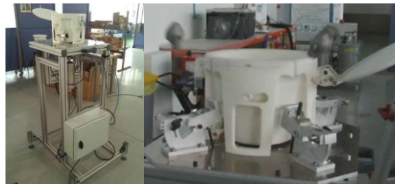
Figure 5 – Complete net launching system (left) and canister container closer view (right)
