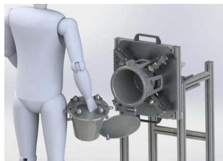
Figure 8 – Operating handling the net reload tool
