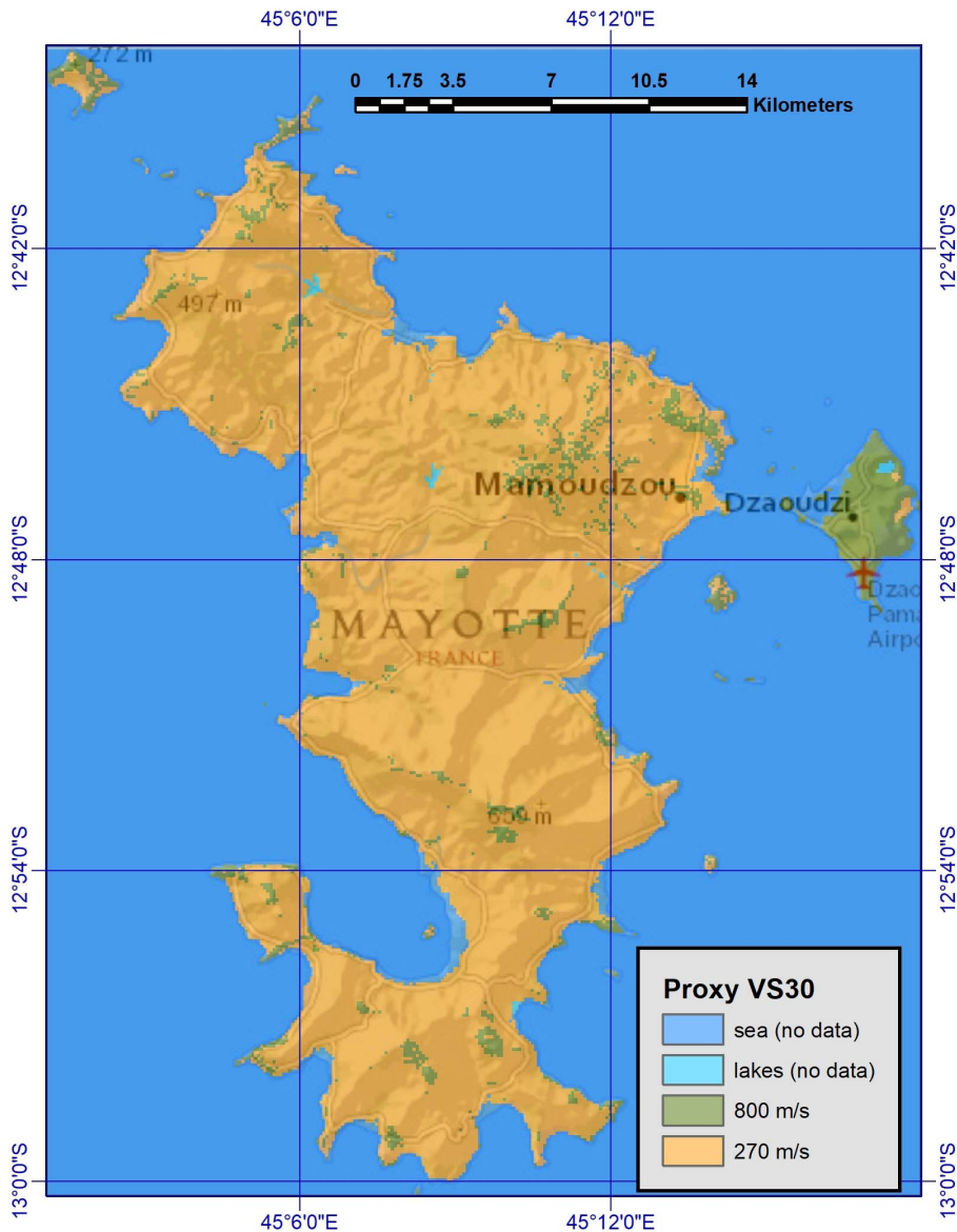
Figure 3. Map of the proxy for the site effects, based on the geological map of Mayotte from Nehlig et al. [2013]. Two soil categories, defined by their mean values of the soil velocity are considered in the calculations.
