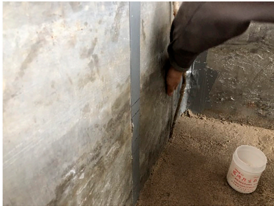
FIGURE 10 Vaseline applied to the wall of the model box.
