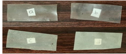
Figure 1. Bioplastic with Al 2 O 3 addition (a) 0%, (b) 1%, (c) 3%, (d) 5%.
