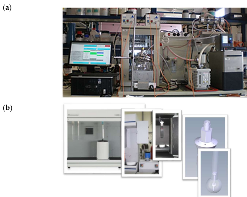
Figure 4. (a) A third-generation calibration system designed by the IC team at the UPNA; (b) a fourth-generation calibration system (adapted from a Micromeritics adsorption device for calibrating an FOS), currently in testing.
