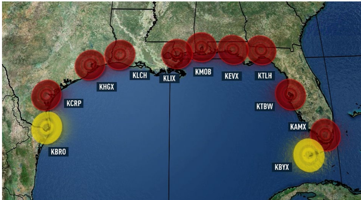
Figure 2. NEXRAD WSR stations along the Gulf of Mexico . Locations of weather surveillance radar (WSR-88D) stations in the immediate proximity of the Gulf of Mexico. Circles depict surveillance radii of 100 kilometers where the beam centers at an altitude of 1,500 meters and samples an area ~1,500 meters in diameter. The Brownsville TX (KBRO) and Key West FL (KBYX) radars are shown in yellow because their data were not used in the analysis.
