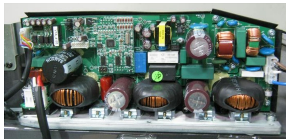
Figure 14 – Exposed view of the drive board used in the SportsArt ECOPOWR G575r Recumbent Cycle (SportsArt, n.d.).
