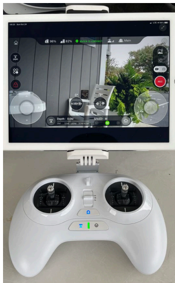
Figure 2c. This is the remote control of the Powervision PowerRay submersible remotely operated vehicle (ROV) and user interface of the Vision+ app which displays the controls, live feed of the video camera, as well as sonar.
