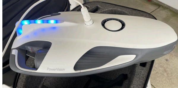
Figure 2a. This is the topside of the Powervision PowerRay submersible remotely operated vehicle (ROV). The power light is on indicating that the tether is connected. Also on the top of the ROV is one of the depth control propellers.
