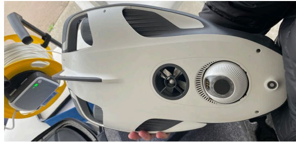
Figure 2b. This is the bottom of the Powervision PowerRay submersible remotely operated vehicle (ROV). The large spherical object visible is the sonar sensor. Also on the bottom of the ROV is one of the depth control propellers.
