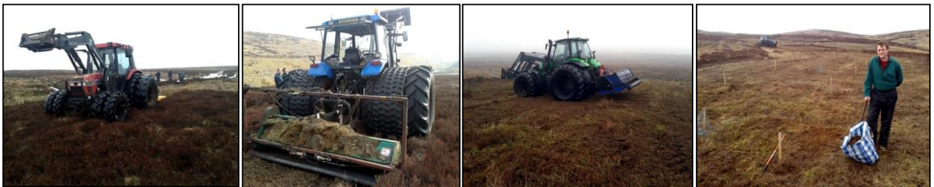
Fig. 6 The three mowing arrangements ( from left to right ): Nidderdale, Mossdale and Whitendale. On average, vegetation was mown about 12 cm above the peat surface and the heather brash returned to the surface was about 5-10 cm long, with the coarsest brash at Nidderdale and the finest at Whitendale. The initial brash layer after mowing was around 5 cm thick. Brash was removed from mown (BR) and mown with added Sphagnum (BRSp) plots by manual raking (~4-5 times ca. 50 L brash were collected from the 5x5 m plots in 70 L bags, see picture on the far right and deposited in adjacent areas.
