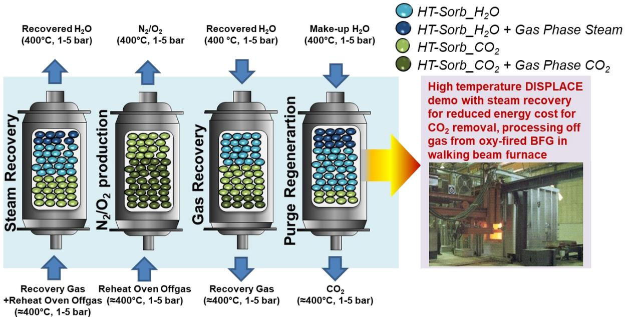
Fig. 2. The general process sequence of stages for the DISPLACE process applied to off-gases from reheating furnaces.
