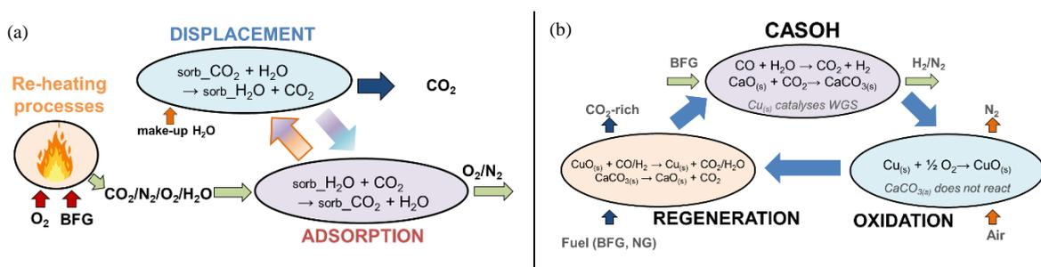
Fig. 1. Conceptual representation of two examples of application of the C<sup>4</sup>U high temperature solid looping technologies for steel mills: (a) DISPLACE; (b) CASOH.
