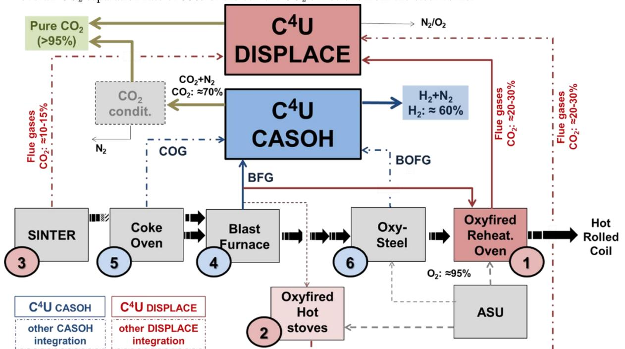
Fig. 9. Block flow diagram of main production units in a steel mill integrated with  $C^4U$   $CO_2$  capture technologies.
