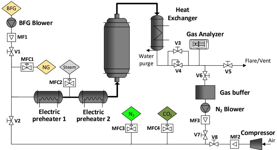
Fig. 7. Simplified process flow diagram of the CASOH pilot.
