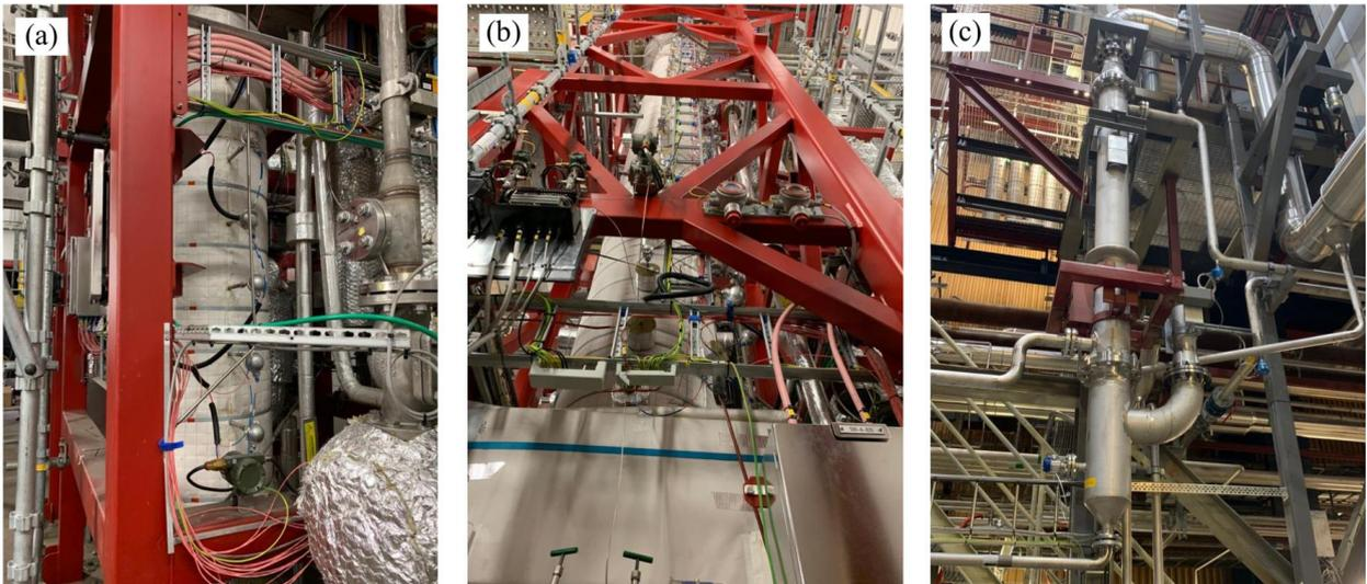
Fig. 5. DISPLACE CO<sub>2</sub> capture equipment: (a) WGS reactor for C<sup>4</sup>U-SEWGS campaign; (b) single column DISPLACE capture unit; (c) syngas cooler.
