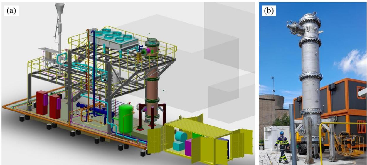
Fig. 8. The main CASOH pilot components: (a) 3D layout of the pilot; (b) the CASOH reactor for TRL7 demonstration.
