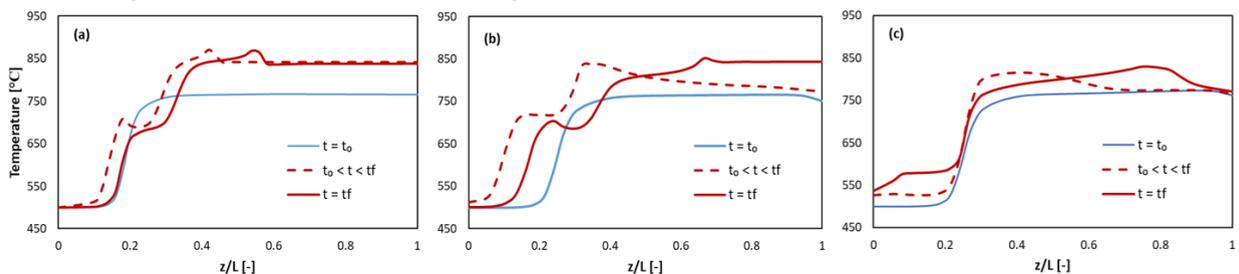
Fig. 14. Evolution of the temperature profiles during the regeneration stage for different regenerative gas mixtures: (a) BFG only; (b) BFG/BOFG/COG; (c) natural gas.
