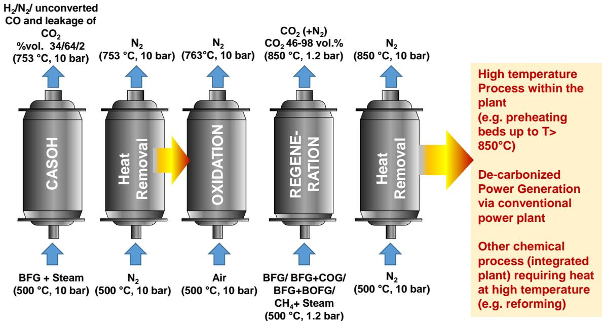
Fig. 6. CASOH scheme reaction network using BFG for both H<sub>2</sub>/N<sub>2</sub> production and sorbent regeneration (other low N<sub>2</sub> content fuel gases such as NG, BOFG and COG can be used in the regeneration stage to further increase purity of CO<sub>2</sub>).
