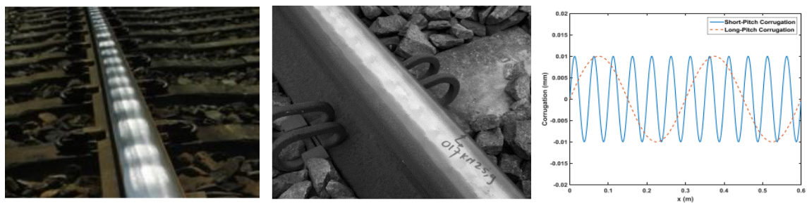
Figure 14. Showing (A) Long-pitch corrugation defect [24], (B) Short-pitch corrugation defect [25], and (C) Short-pitch and long-pitch corrugation [26].
