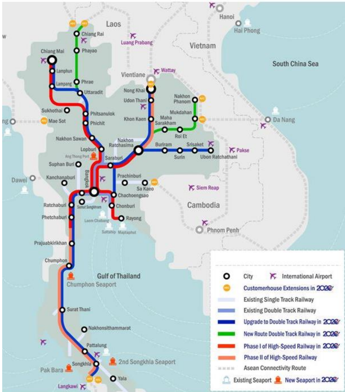
Figure 1. A high-speed train project is planned to operate in Thailand, which consists of 4 main lines. Starting from Bangkok to Chiangmai, Nong Khai, Rayong and Padang Besar (Malaysia) with a 250 km/hr speed for a distance of 1,039 km.
