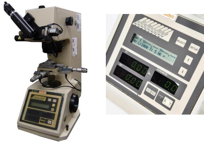
Figure 58. Micro Vicker hardness tester Mitutoyo MVK-H1 [111].
