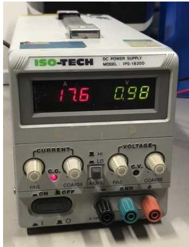
Figure 93. DCPD instrument (Left) and a cracked material in the DCPD testing (Right).
