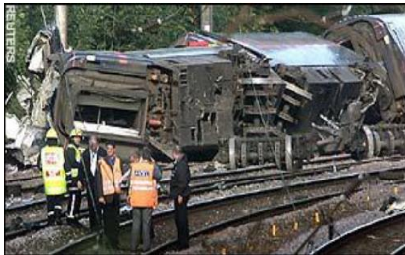
Figure 28. A high-speed train had a catastrophic fatigue breakdown south of Hatfield station in the United Kingdom (October 2000) [27].
