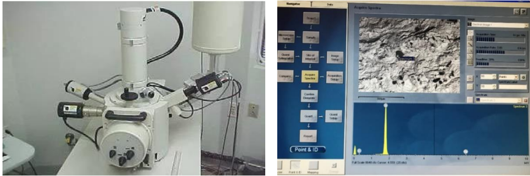
Figure 95. SEM JEOL 6060 with EDS Unit Overview.
