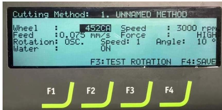
Figure 78. The parameter used for cutting the Hadfield manganese steel.
