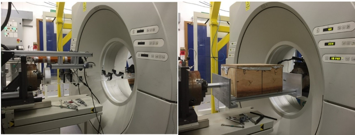
Figure 3-18 Scanning of block C3 in a medical level X-ray scanner: normal set-up for small cylindrical samples (left) and modified set-up for large soil blocks (right)
