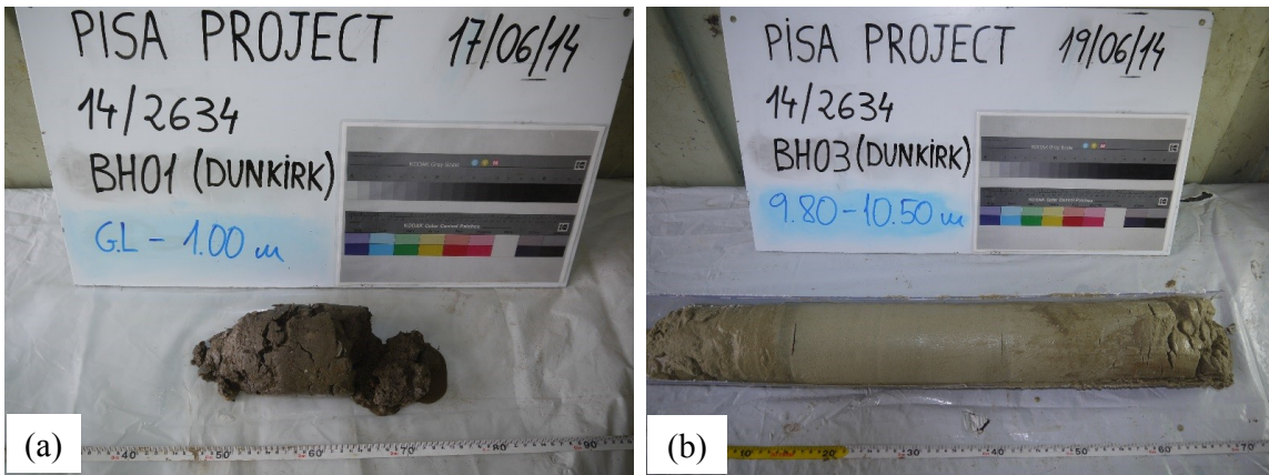
Figure 2-7 Examples of drilled (a) poor quality and (b) promising ‘intact’ cores retrieved from the PISA rotatory core sampling campaign at the Dunkirk site
