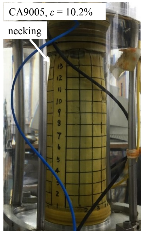
Continued Figure 3-38 Deformation pattern and failure mode of the HCA samples at ultimate shearing strains \epsilon ( = \epsilon_1 - \epsilon_3 )
