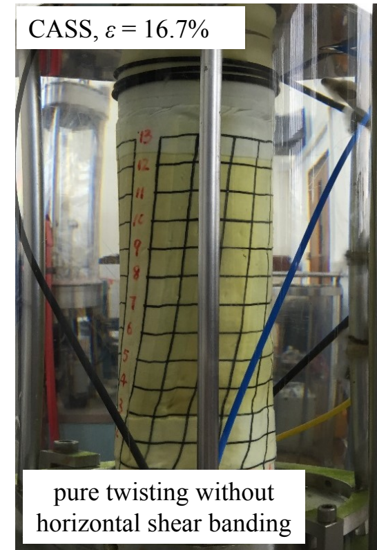
Figure 3-38 Deformation pattern and failure mode of the HCA samples at ultimate shearing strains \varepsilon ( = \varepsilon_1 - \varepsilon_3 )
