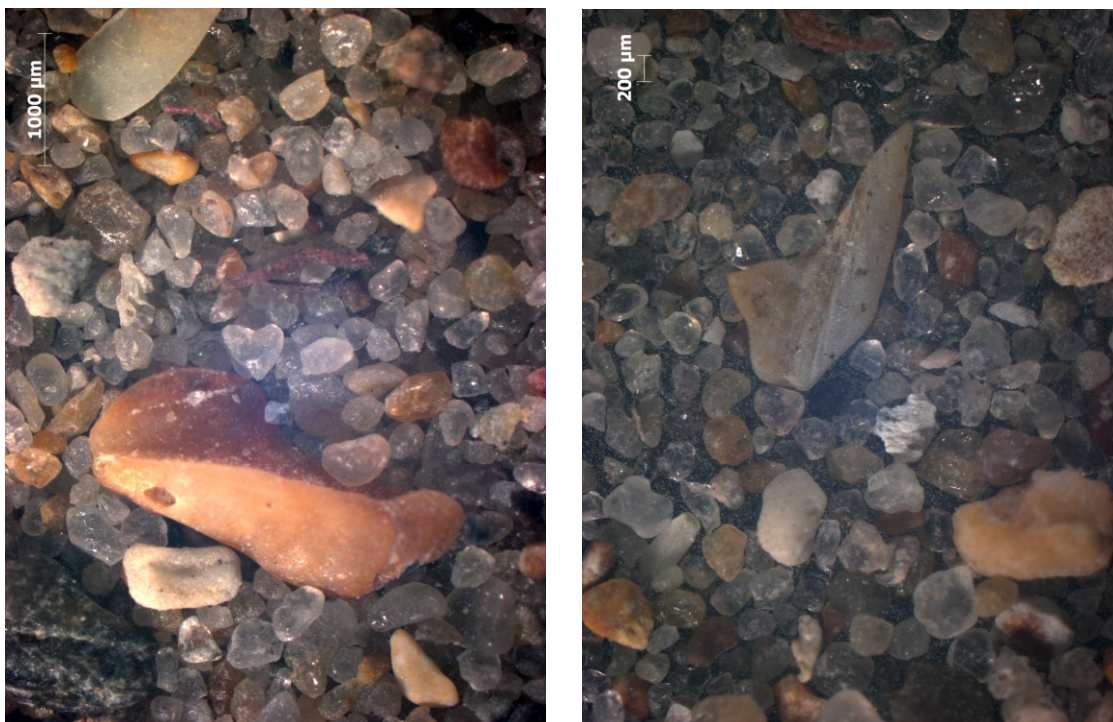
Figure 4-18 Optical microscope images of dry Dunkirk sand Batch 2, featured with elongated shell fragments and grains of varied shape, size and colour
