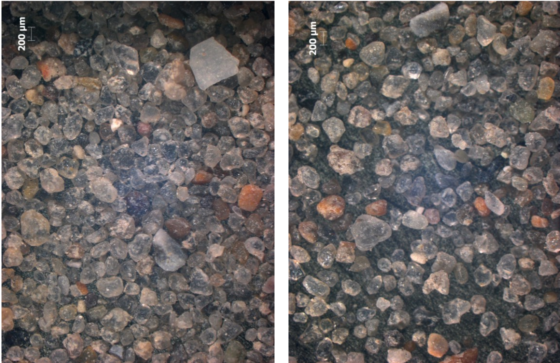
Figure 4-19 Optical microscope images of dry Dunkirk sand Batch 3, identifying mixed grains of varied origins and less reflective grains surfaces compared to the Batch 2
