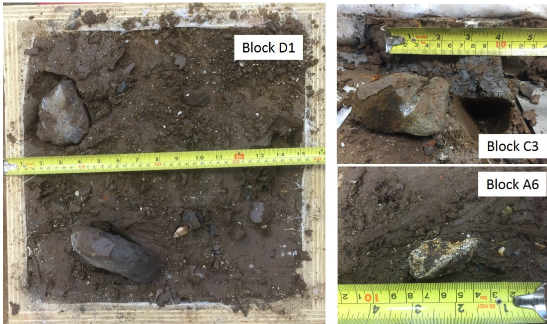
Figure 3-13 Examples of large hard inclusions encountered in Cowden till block samples
