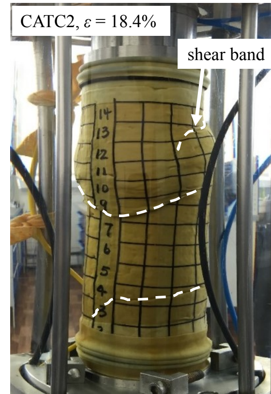
Continued Figure 3-38 Deformation pattern and failure mode of the HCA samples at ultimate shearing strains \epsilon ( = \epsilon_1 - \epsilon_3 )
