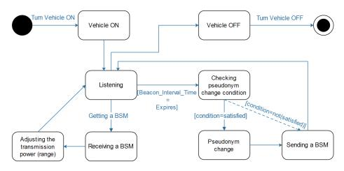
Figure 6. The state diagram of WHISPER.
