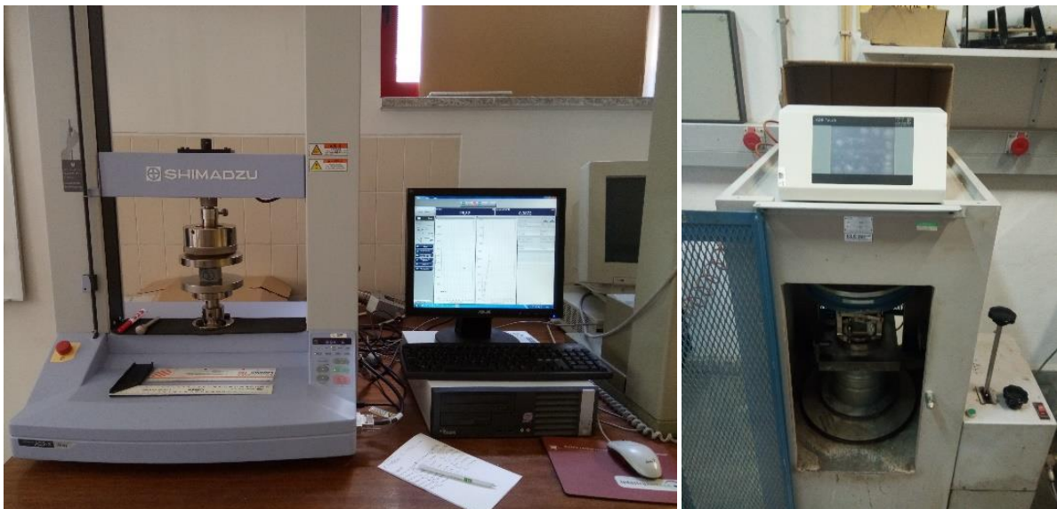
Figure 3.13 - Machines used for the compressive strength test ( left ): Autograph AGS-X, 10 KN SHIMADZU, ( right ): ADR Touch ELE international limited.
