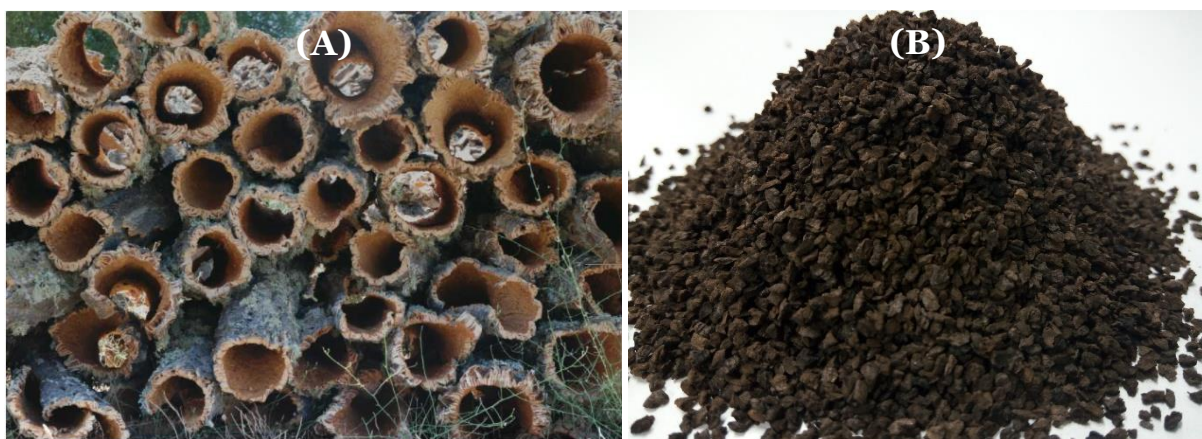
Figure 2.12 - Cellular structure of natural Cork (A) and (B): cork particles
