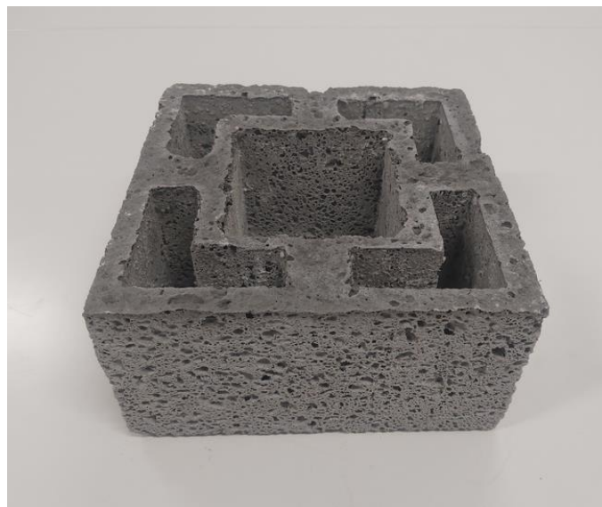
Figure 4.8 - Perforated prototype block (Cobogós) tungsten-based obtained by expansion inside the mould.
