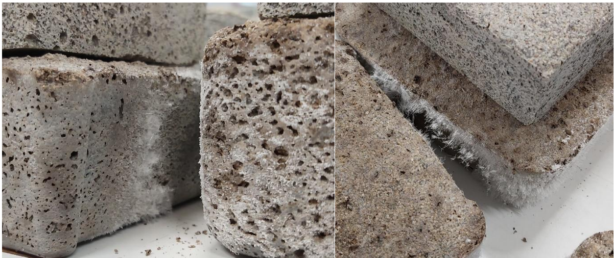
Figure 4.11 - AALWF-Mortar samples under the efflorescence phenomena.
