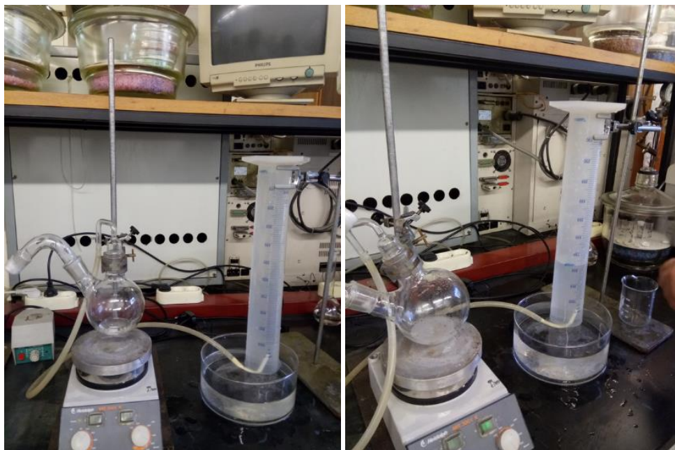
Figure 3.10 - Setup to measure the H 2 volume released of Al powder reaction with a 10 M NaOH solution.
