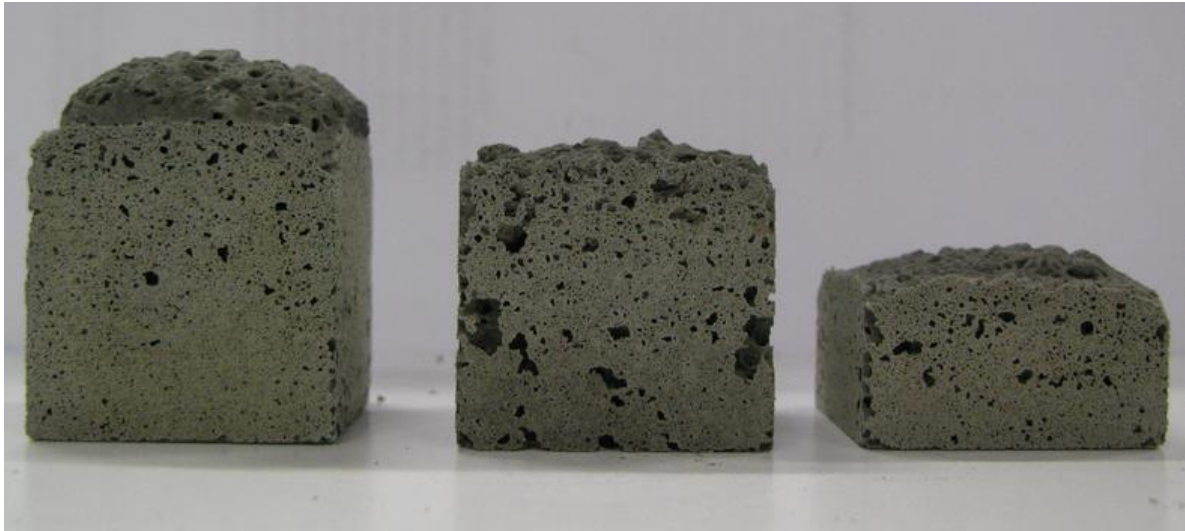
Figure 5.3 – Photograph of the preliminary alkali-activated binders with cement mixtures foamed with Al powder.
