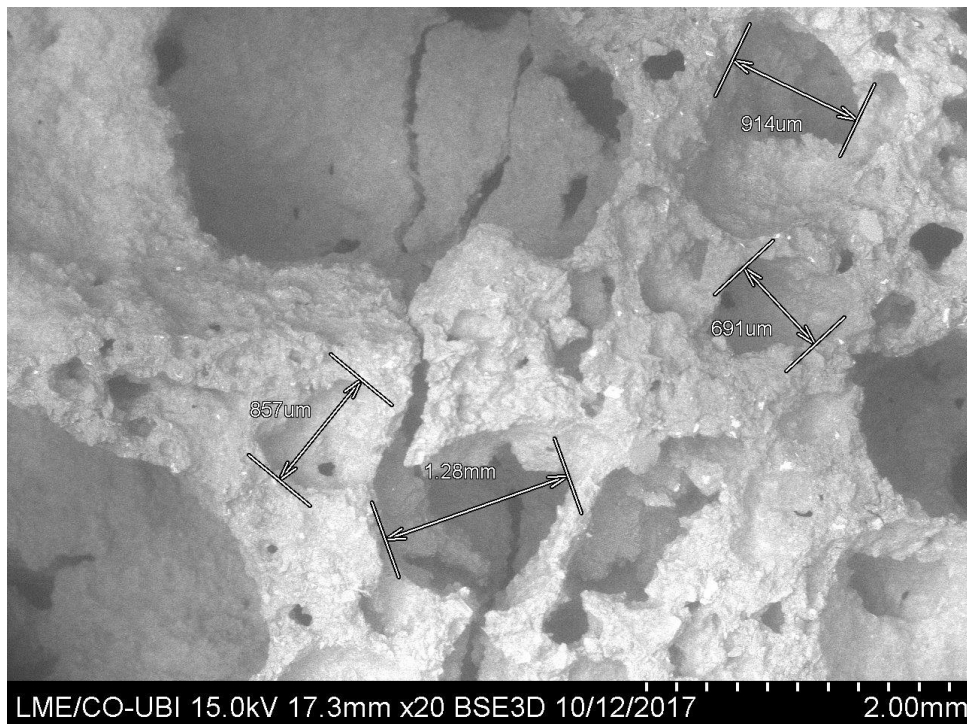
Figure 4.6 - SEM images of the highly porous structure of the alkali-activated foams binder.
