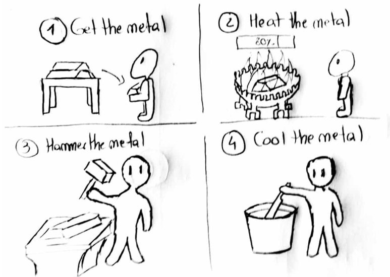
Figure 3.27: Process of forging a blade
