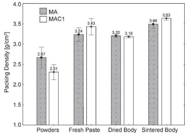
Fig. 6. Changes in particle packing density in compositions MA (no cement) and MAC1 (1 wt.% CAC): dry loose powders, fluid fresh paste, dried hardened body and sintered body (mean value \pm 0.95 confidence interval).
