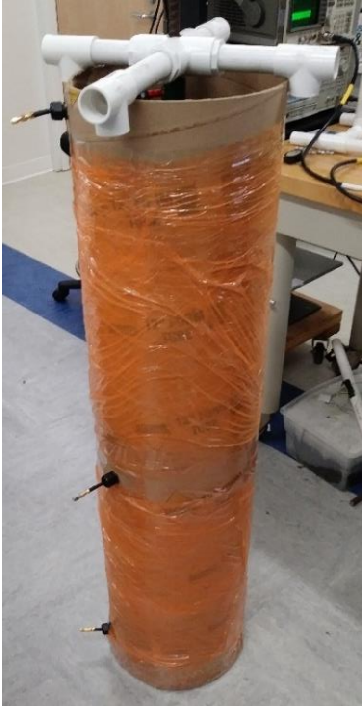
Figure 26. Experiment 6 concrete form during curing.
