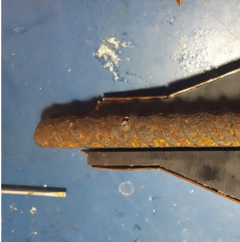
Figure 6. Machine screw through drilled hole in rebar.
