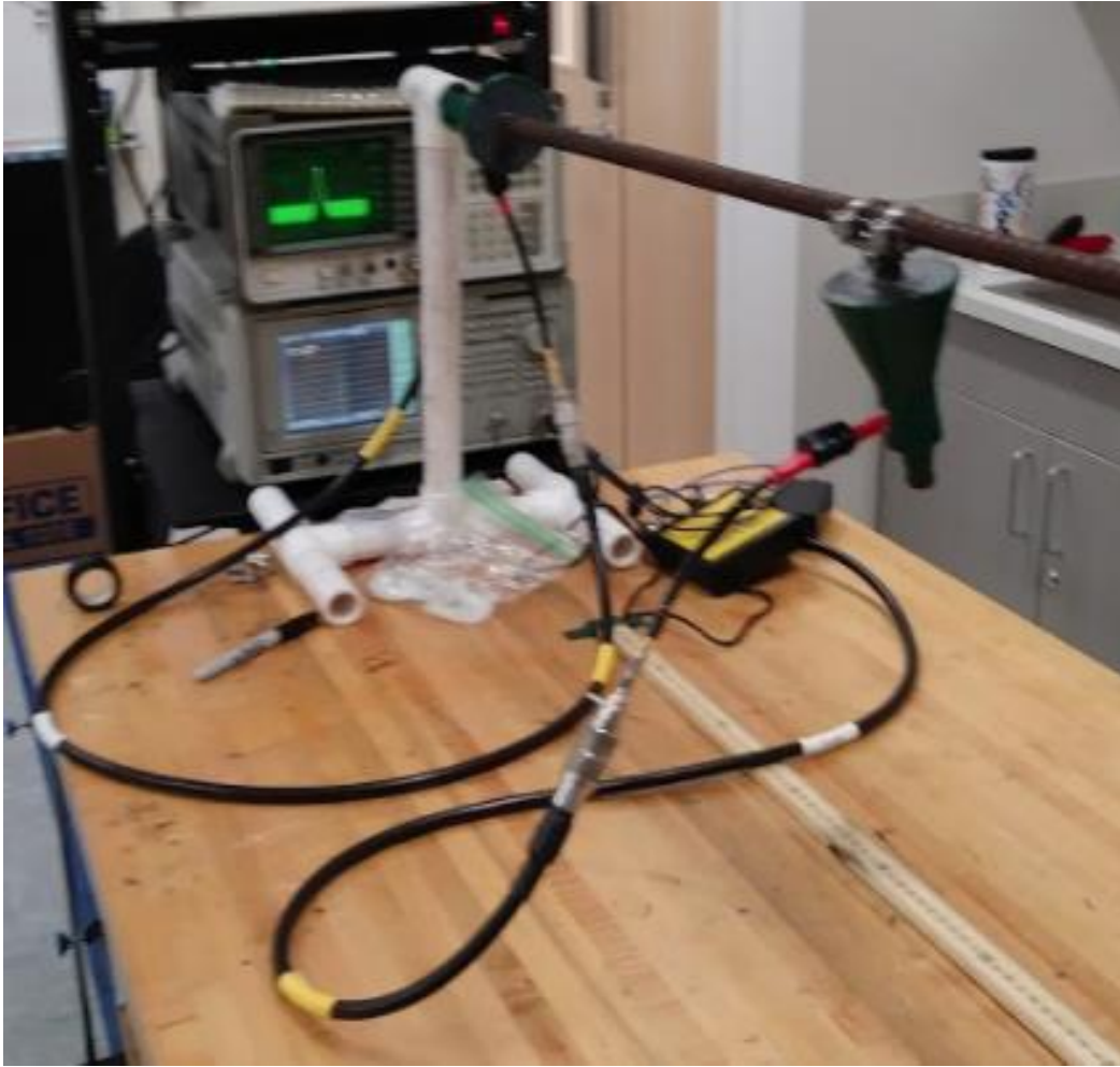
Figure 19. Experiment 4 inline and perpendicular receive couplers.
