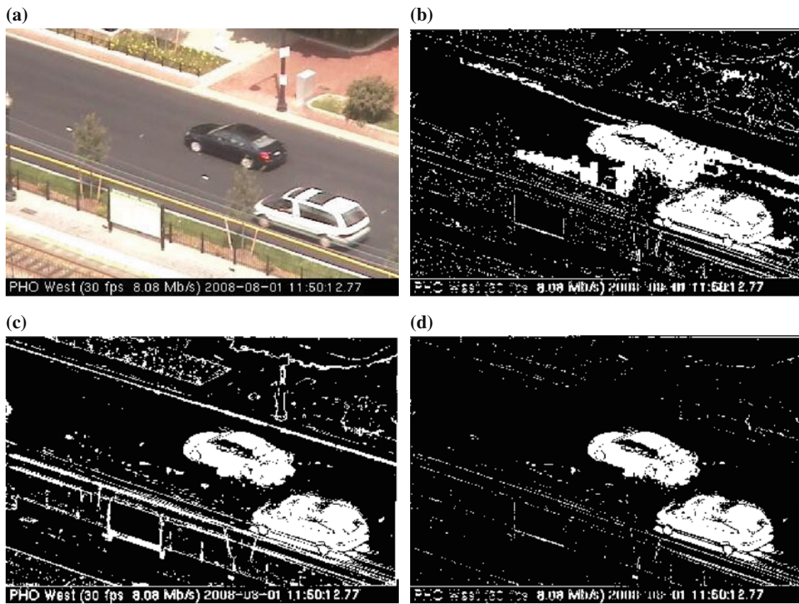
Fig. 5 Example of background subtraction with the Temporal, the Spatio-Temporal and our approach, which combines the two. This figure gives an idea of the complementarity of the foreground mask resulting from the Temporal and the Spatio-Temporal approaches on the frame (a). The Temporal approach in b estimates a noisy and sparse foreground. Instead, the Spatio-Temporal background subtraction output in c is cleaner and the region classified as foreground is thick. If we combine the two results with a binary AND, we obtain that the noisy
