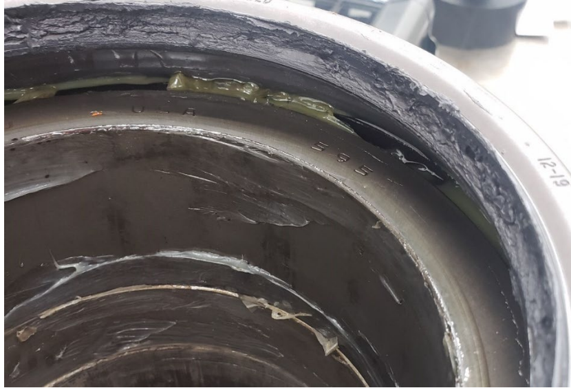
Figure 7. Rubbing Lip Seal Bearing at the End of Environmental Test
