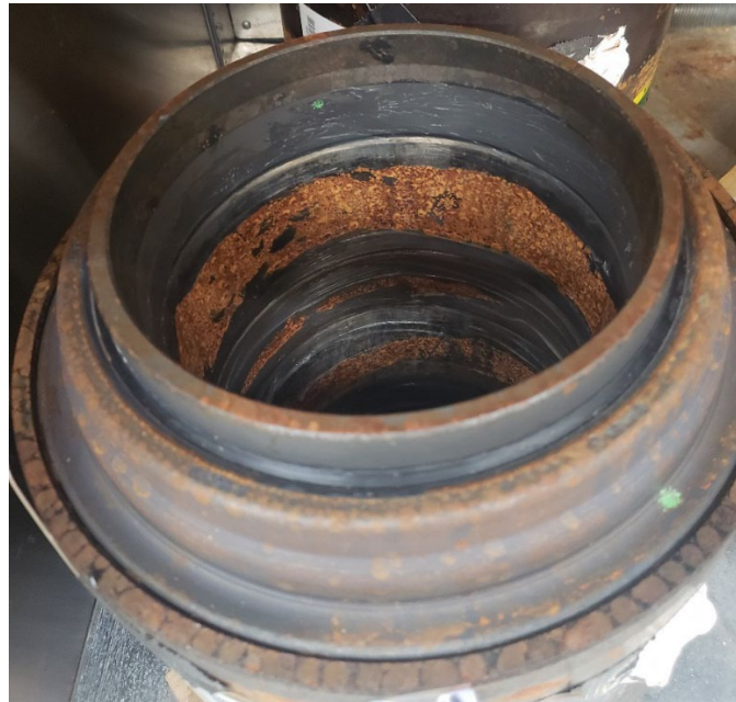
Figure 5. Corrosion on Bearing Surfaces
