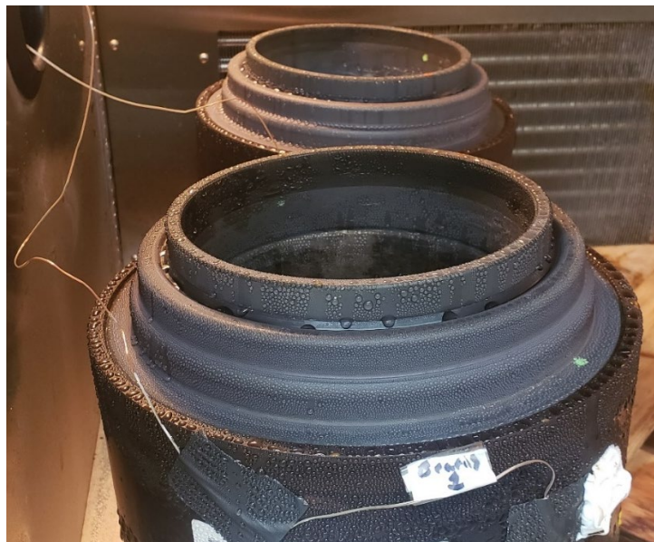
Figure 4. Bearings in Environmental Chamber
