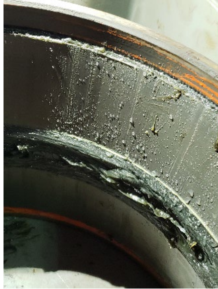
Figure 1. Bearing Cup Running Surface with Water Ingress
