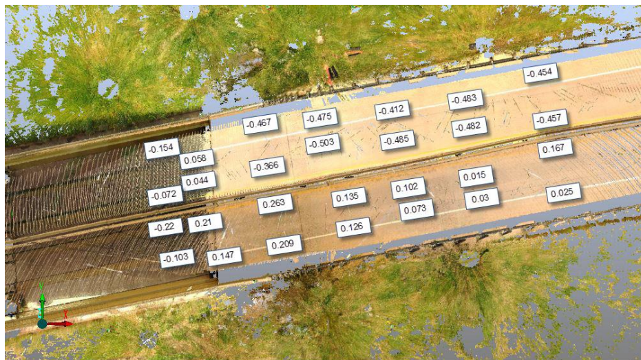
Figure 15. Cumulative total vertical deformations from April 2016 to July 2016
