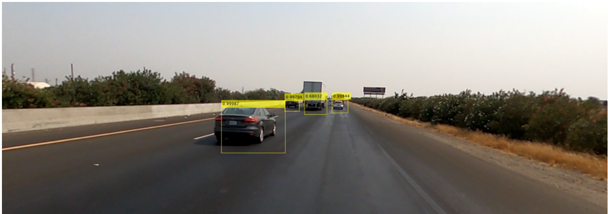
Figure 7. An Illustration of Vehicle Detection
