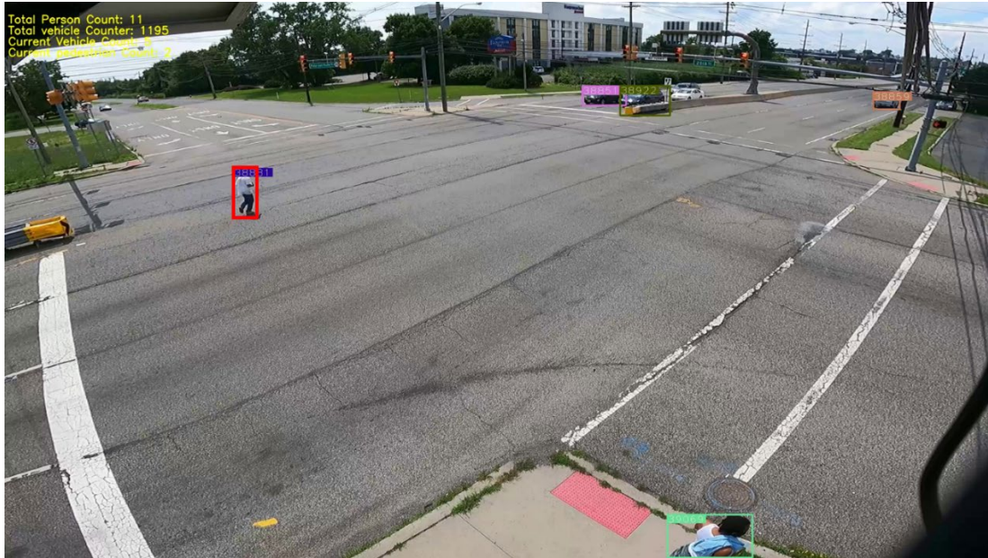
Figure 33 An illustration of the detected pedestrian non-compliance event
