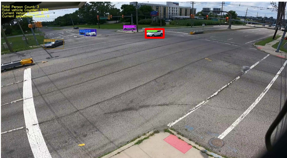
Figure 32 An illustration of the detected vehicle non-compliance event
