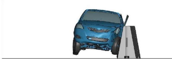
b. t = 0.23 s, event = rear right tire contacts the barrier, window pane snags against the barrier
