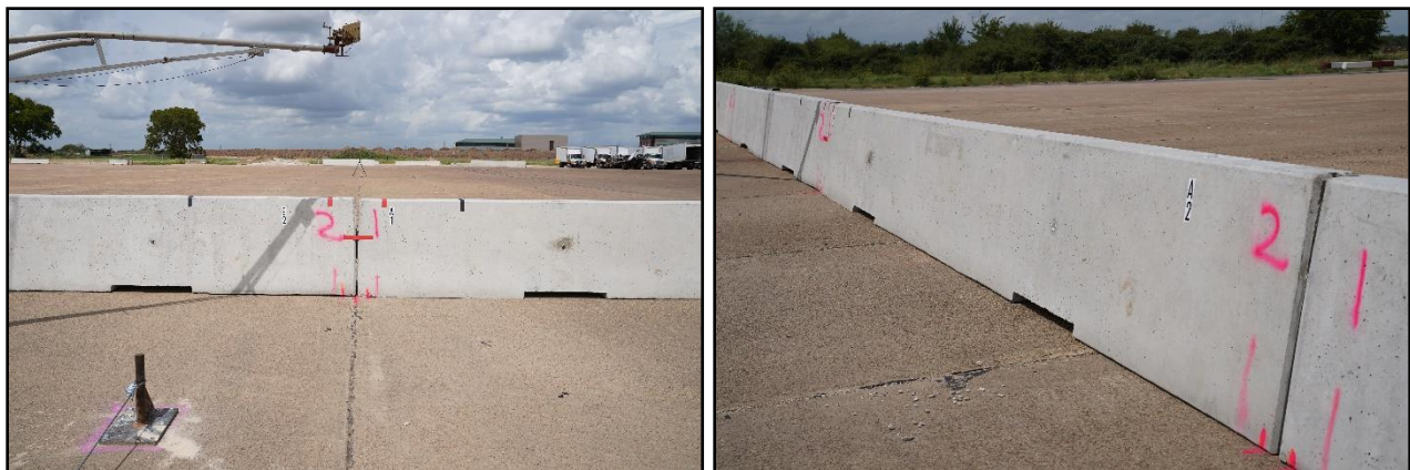
Figure 5.10. Single-Slope Barrier prior to Test No. 440591-01-B2.
