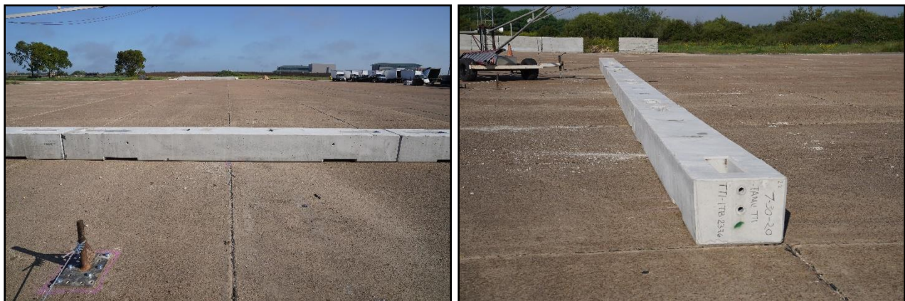
Figure 6.1. Low-Profile Barrier prior to Test No. 440591-01-B5.
