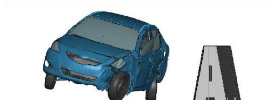
e. t = 0.91 s, event = rear right tire stabilizes on ground
