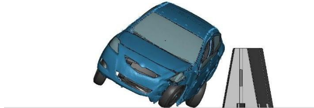
d. t = 0.62 s, event = rear right tire touches ground
