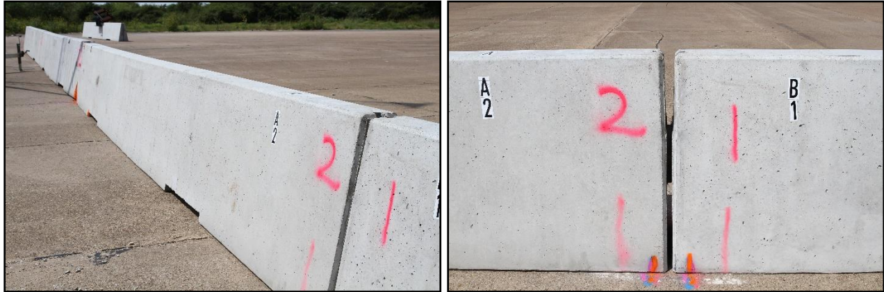
Figure 5.22. Single-Slope Barrier prior to Test No. 440591-01-B10.
