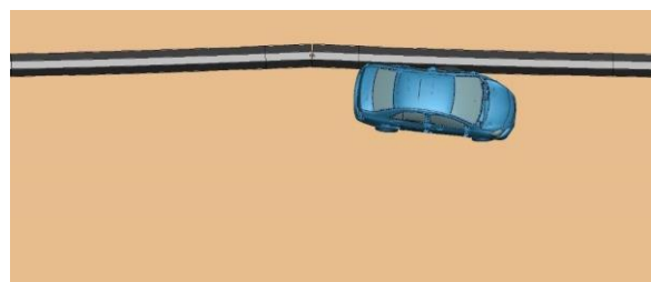
c. t = 0.33 s, event = car redirected by the barrier
