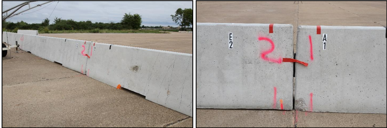
Figure 5.14. Single-Slope Barrier prior to Test No. 440591-01-B9.
