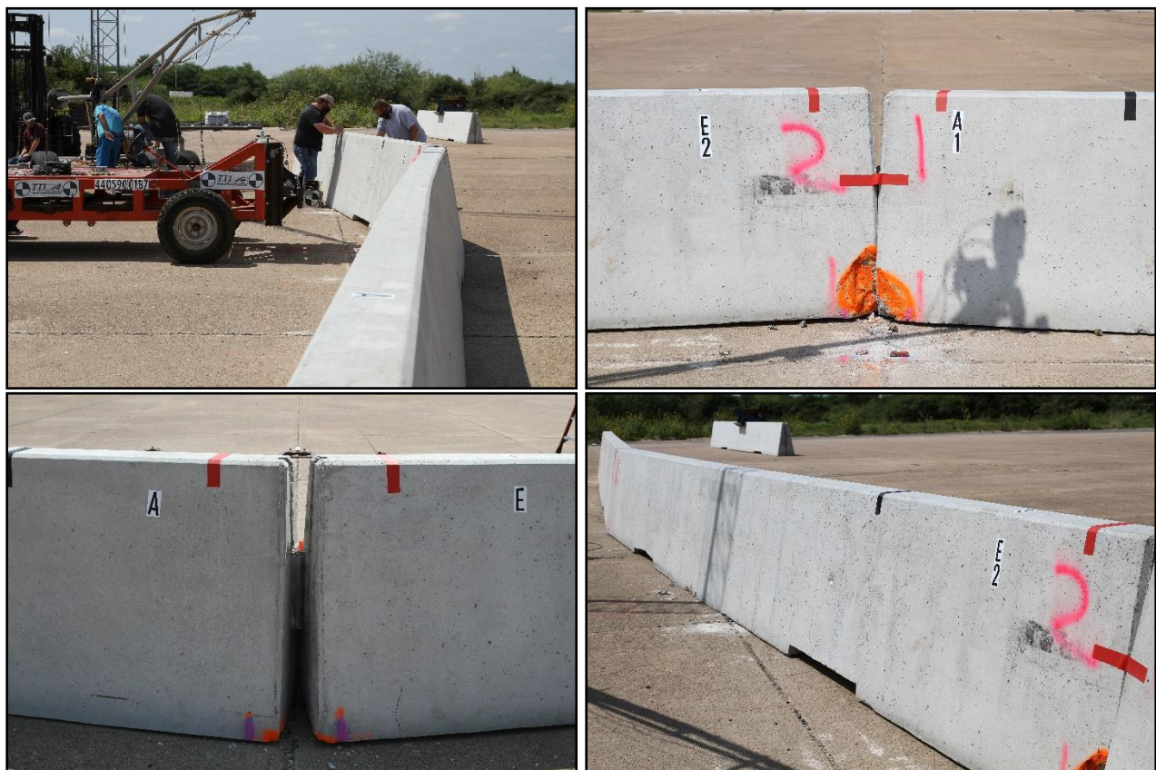
Figure 5.20. Single-Slope Barrier after Test No. 440591-01-B7.
