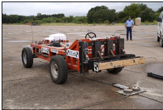
Figure 5.1. Surrogate Test Vehicle for Single-Slope Barrier.
