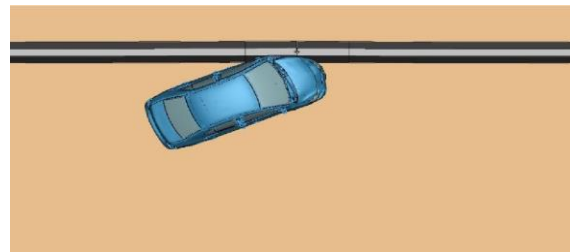
b. t = 0.13 s, event = car contacts the joint
