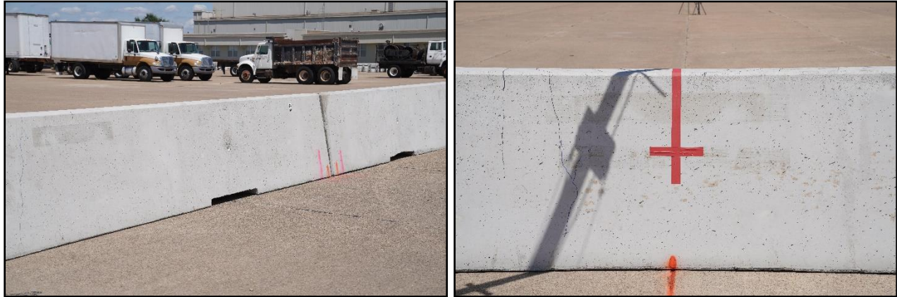
Figure 5.6. Single-Slope Barrier prior to Test No. 440590-01-B8.
