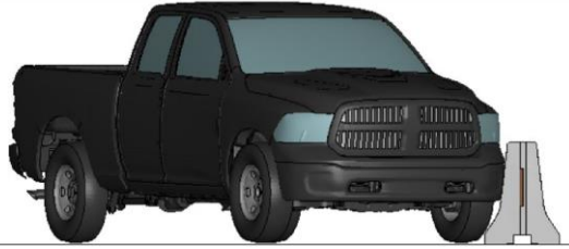
a. t = 0.10 s, event = front right tire contacts the barrier
