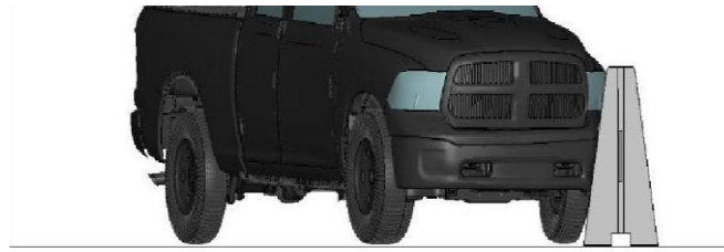
a. t = 0.10 s, event = front right tire contacts the barrier
