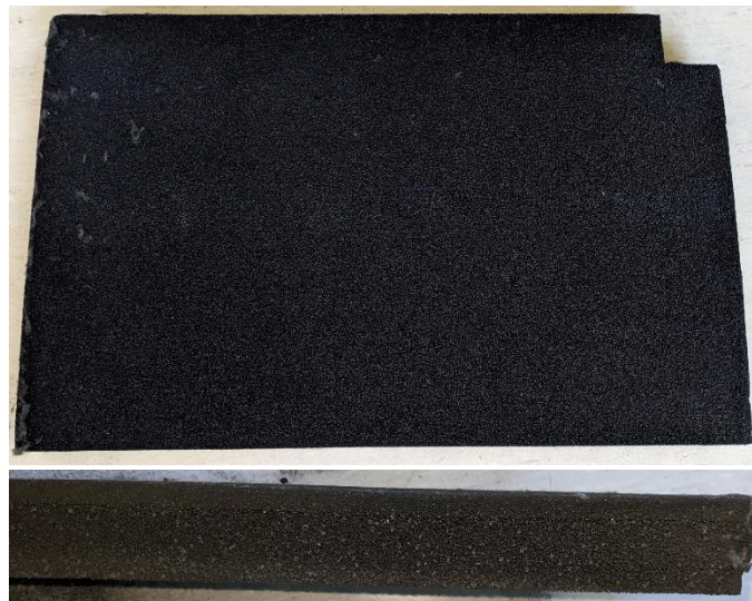
Figure 2: MERV-8 foam filters, 15.25x19.25x1.75 inches
