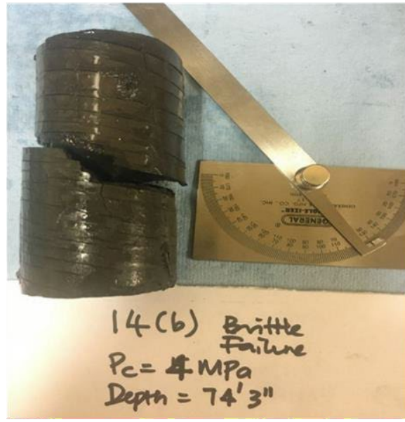
(b) Sliding failure along discontinuities
