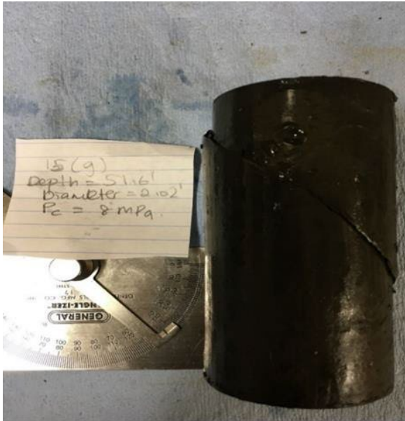
(a) Sliding failure across discontinuities
