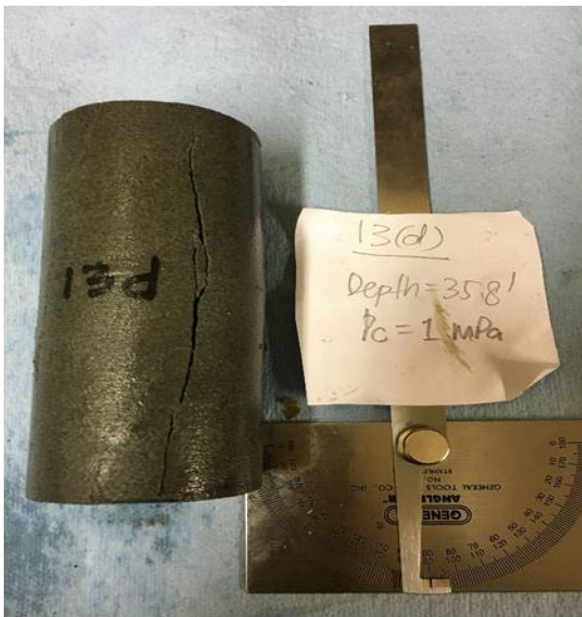
(c) Tensile failure across discontinuities
