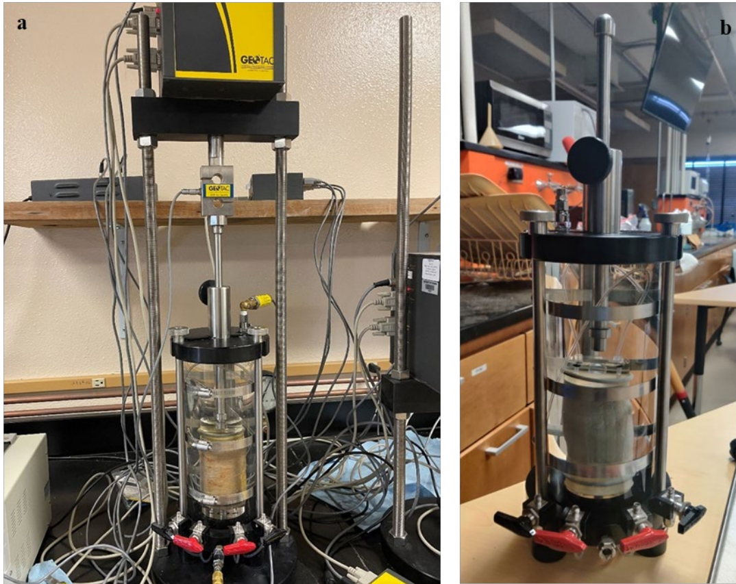
Figure 3.14 Application of axial load during the shearing stage (a) and final deformed shape of the specimen (b)
