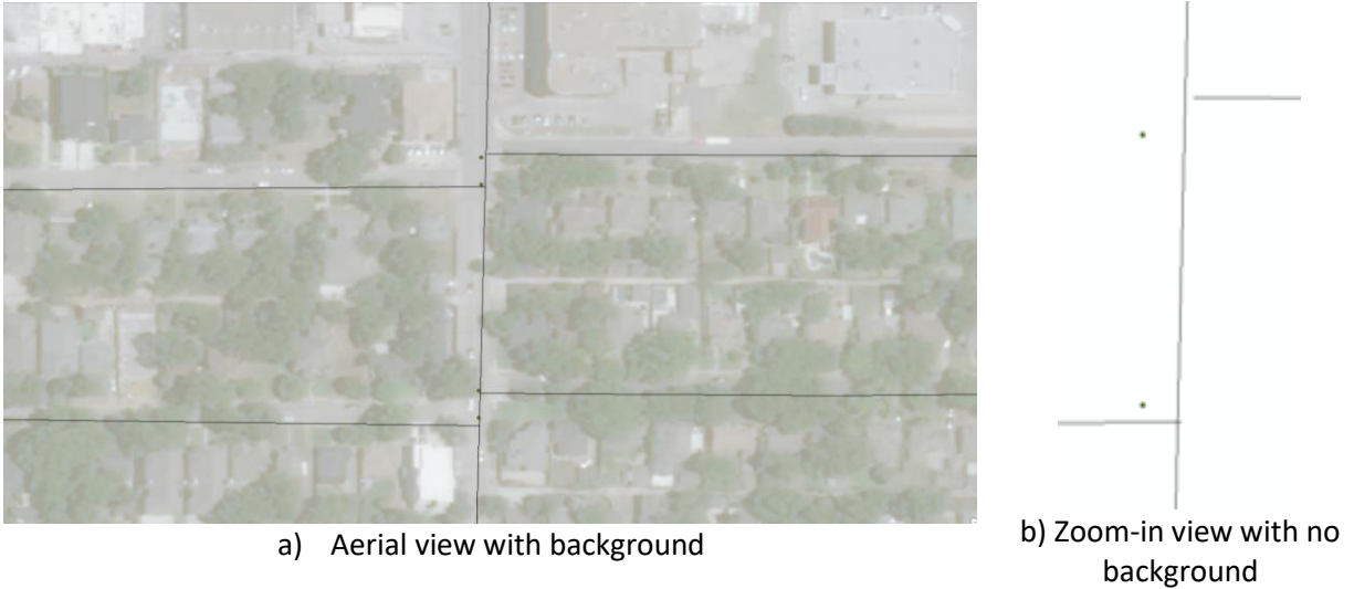
Figure 15. Offset between Road Lines and Intersection Points.
