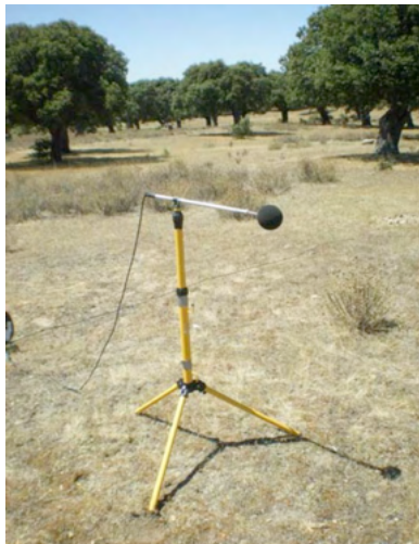
Figure 6. Representative image from the BANOERAC report (2009) showing the ground conditions and the microphone at 1.2 m.
