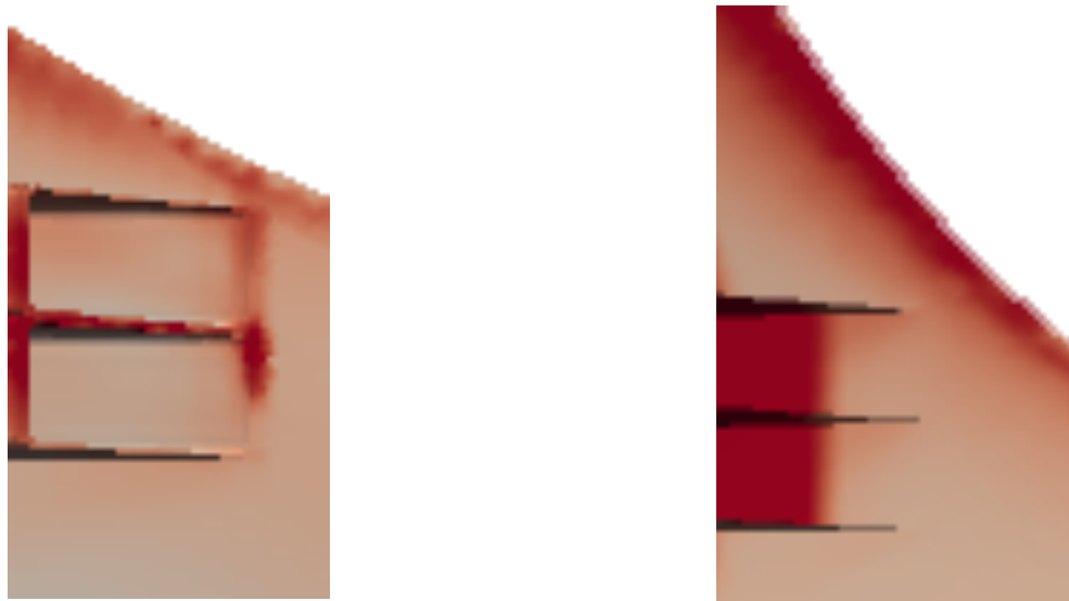
Figure 24. Comparison between the initial nacelle-wing integration (left) and Improved nacelle-wing integration (right).
