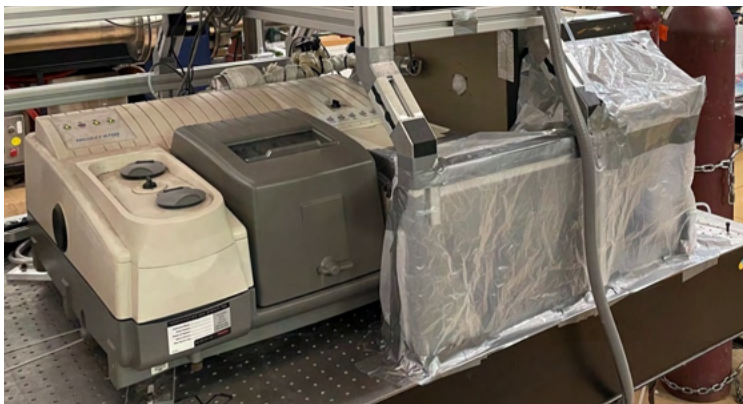
Figure 1. The modified FTIR spectrometer facility, with a purge system constructed to enable purging of the entire optical path length with nitrogen gas during measurements.
