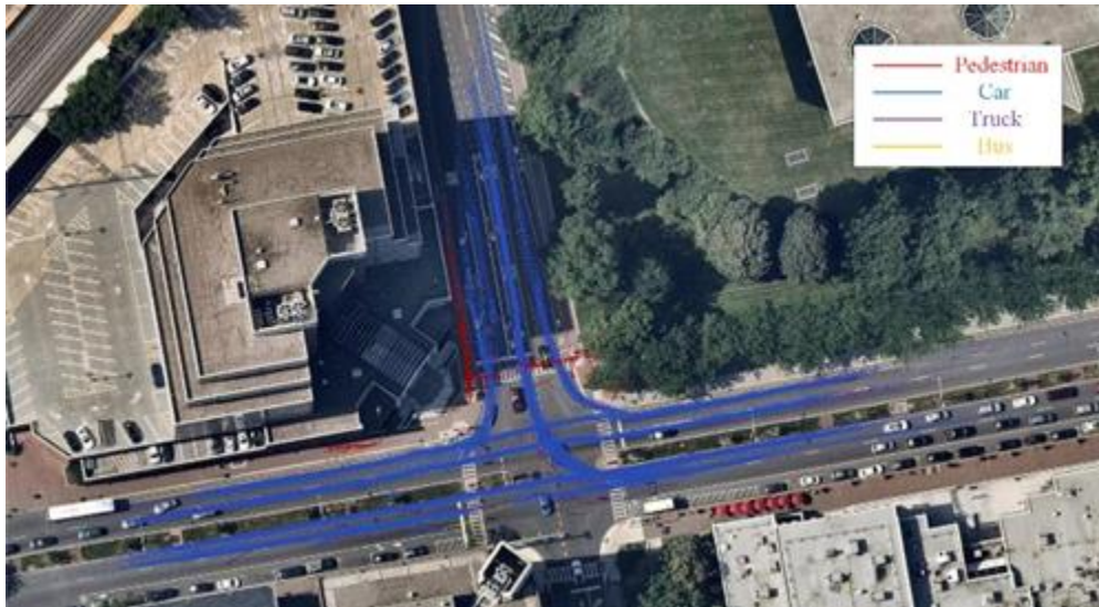
Figure 10. LiDAR Trajectory for Connected Vehicle Applications
