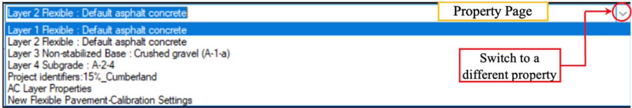
Figure 16. Example of different item properties that typically appear in the Property Page
