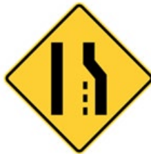
Figure 2. Illustration. Symbolic lane-reduction warning sign, W4-2 (FHWA 2009).
