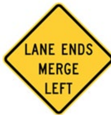
Figure 3. Illustration. Text lane-reduction warning sign, W9-2 (FHWA 2009).
