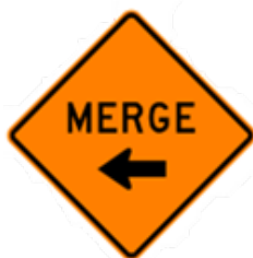
Figure 5. Illustration. Lane-reduction transition sign W20-X3 used in Iowa (Iowa DOT 2017).
