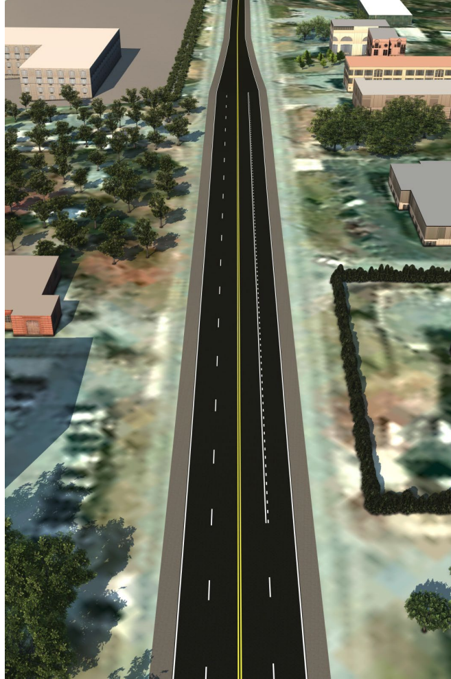
Figure 9. Screenshot. Dotted-line-plus-solid-white-line lane-reduction transition marking.
