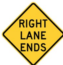
Figure 4. Illustration. Optional additional advance lane-reduction transition sign, W9-1 (FHWA 2009).
