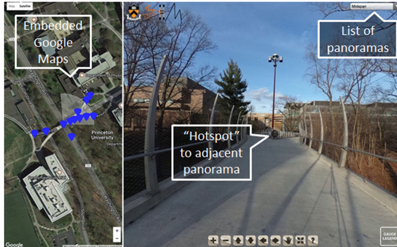
Figure 4: Virtual tour interface illustrating the different types of navigation: (1) embedded Google Maps, (2) “hotspot” connections to adjacent panoramas, and (3) drop-down menu with list of all panoramas of the bridge [3].
