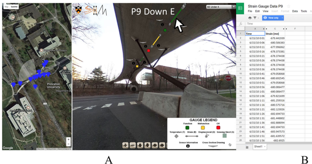
Figure 5: A) When a user hovers over a sensor, they can see its ID as well as what it is measuring. B) When a user clicks on the sensor they can access a database with time series [3].
