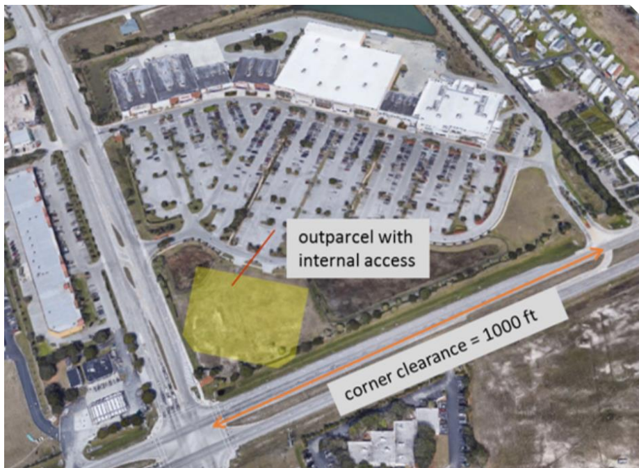
Figure 4: Corner clearance of shopping center access.
