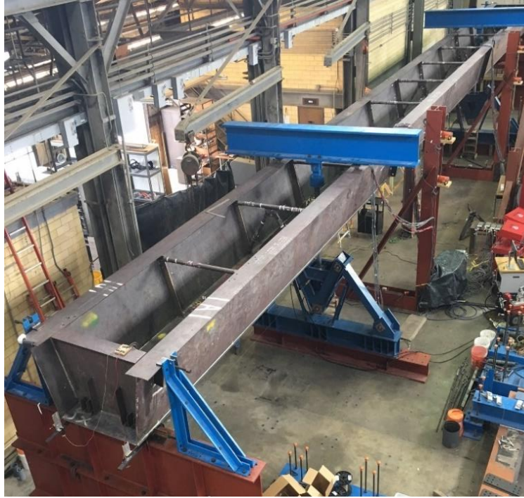
Figure 3-3 –Steel Tub Girder - Test Setup
