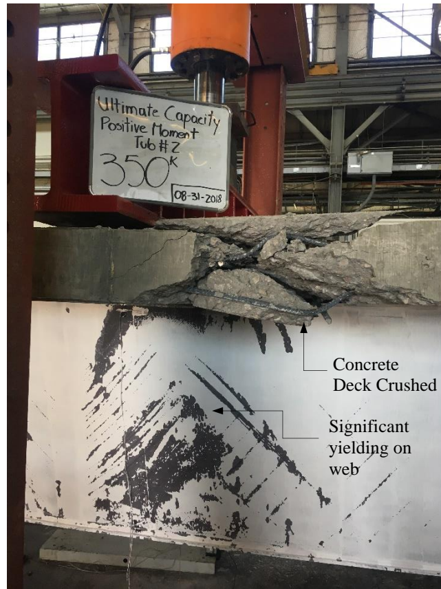
Figure 5-33 - Concrete Deck Crushed and Top Web Buckled – Tub #2
