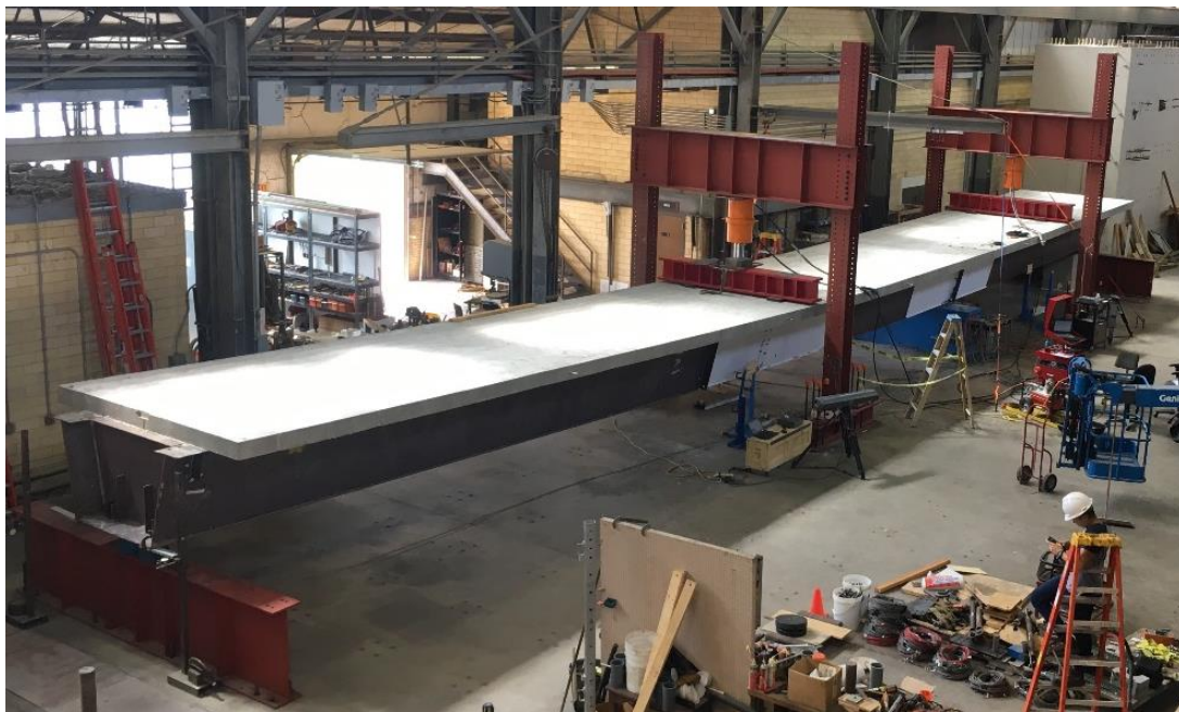
Figure 5-18 - Continuous Girder Test Setup - Tub #1
