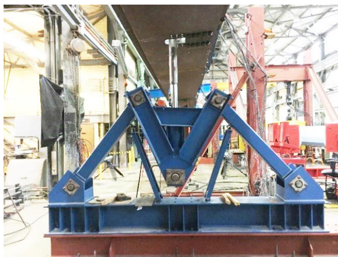
Figure 3-7 - Gravity Load Simulator (GLS) during test
