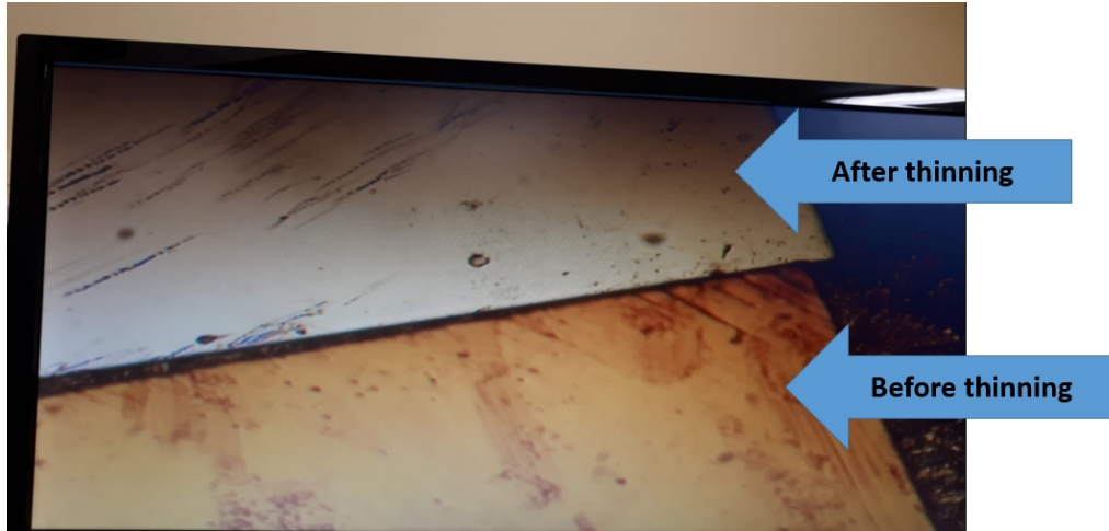
Fig. 3.8: The view of the back side of UFSD3 under the microscope before and after thinning which emphasizes the removal of the metallization layer.
