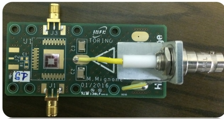
Fig. 3.16: Two channels passive board made by INFN Torino. In this case at most 2 pads from 4 pads UFSD can be connected.
