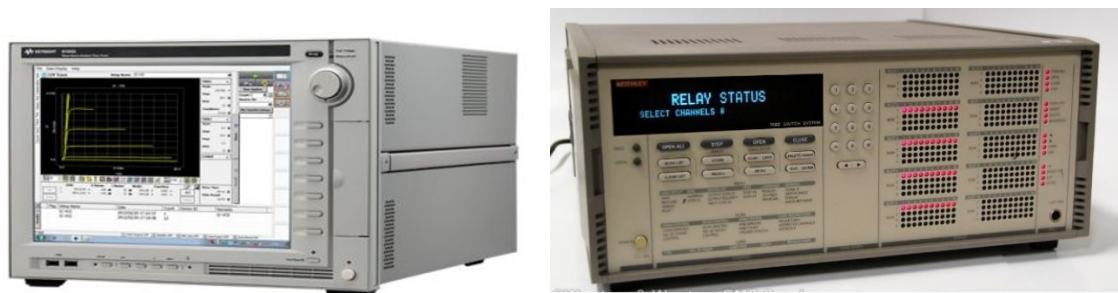
Fig. 3.2: Left: Keysight Technologies Source/Measurement Unit (SMU), Right: switching matrix.
