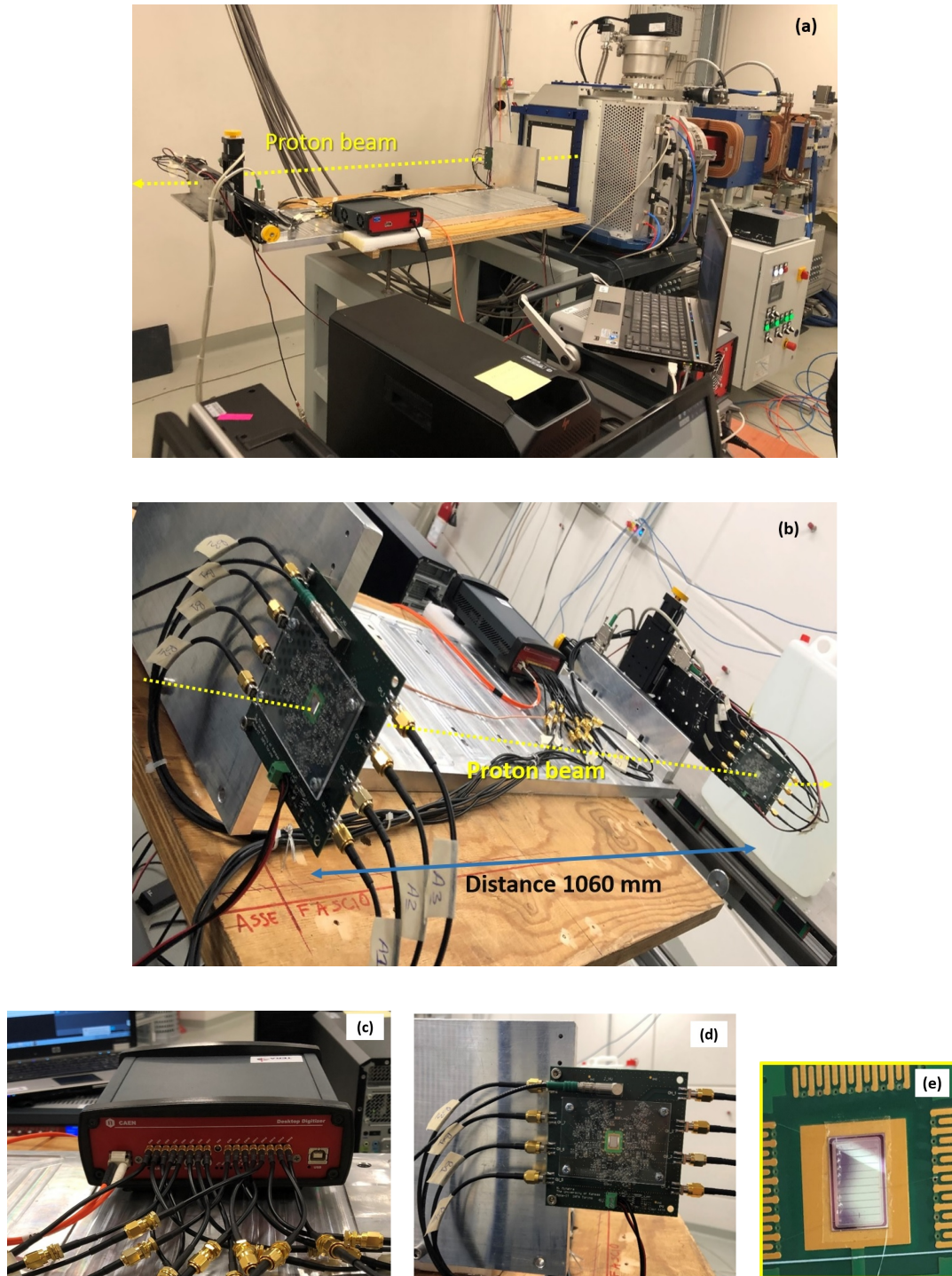
Fig. 4.8: The setup of data acquisition from a beam test performed at CNAO. (a) General view of all setup, the yellow arrow shows the beam direction, (b) The telescope of the sensors in distance 1060 mm, (c) The digitizer with 16 readout channels to collect the data from 8+8 strips, (d) the front-end read out board, and (e) the thinned sensors segmented to 11 strips.
