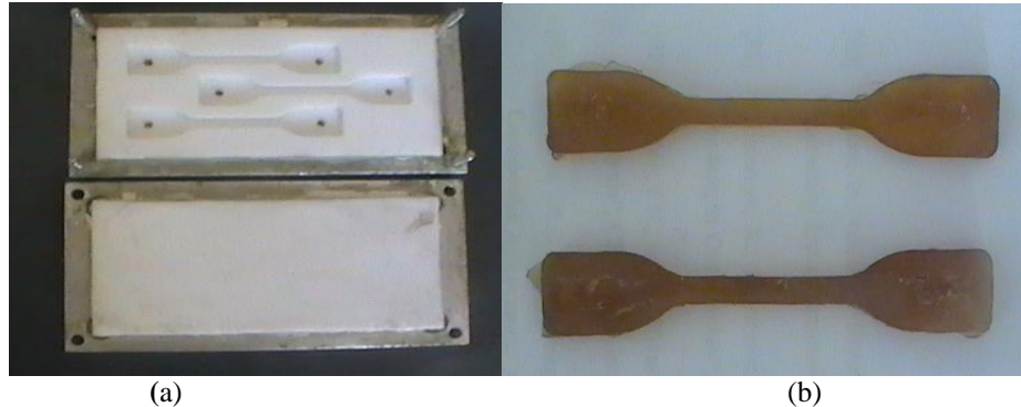
Fig. 1. Bulk adhesive samples: (a) Teflon adhesive mould; (b) sample of hot-melt adhesive specimens
