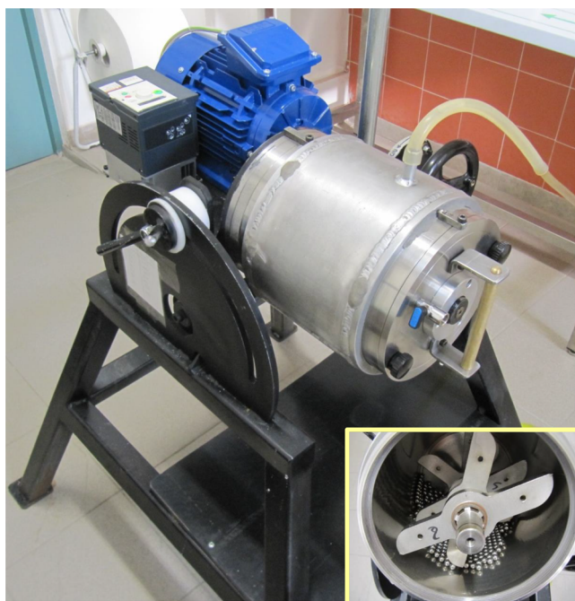
Figure 2. 5 L milling-drum prototype.
