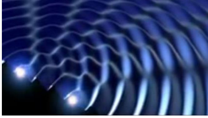
Figure 11. X-rays are scattered by the two atoms (bright spots in the left bottom corner). Interference occurs forming destructive (black) and constructive (bright) zones.
