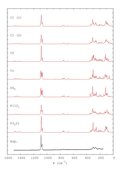
Figure 2 Calculated and experimental Raman spectra of vaterite: expansion of the 1160-1020 cm<sup>-1</sup> range ( $v_1$  modes).
